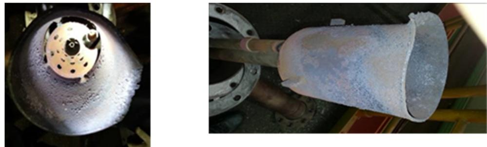
**Figure 5.** An example of the combustion chamber deformation by flame.
