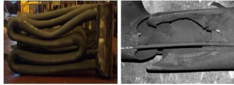
Figure 1. Deformation of radiant tube and combustor.
