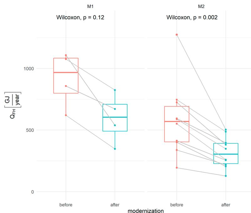
**Figure 1.** Decrease in final energy consumption for heating  $Q_{\text{FH}}$ .
