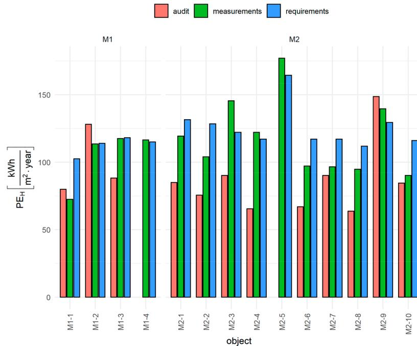
**Figure 5.** Comparison of the obtained  $PE_H$  index values with those calculated in the audit after thermal refurbishment and with the technical requirements.
