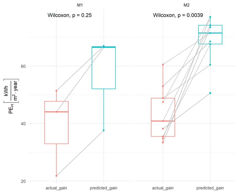
**Figure 3.** Decrease in the value of the  $PE_H$  index calculated on the basis of measurements from the operation of buildings and indexes calculated on the basis of audits.
