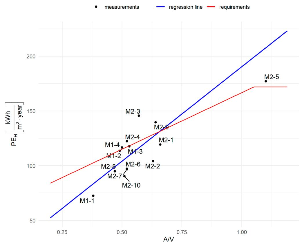
**Figure 6.** Comparison of the obtained mean  $PE_H$  values with the boundary  $PE_{H,0}$  value.
