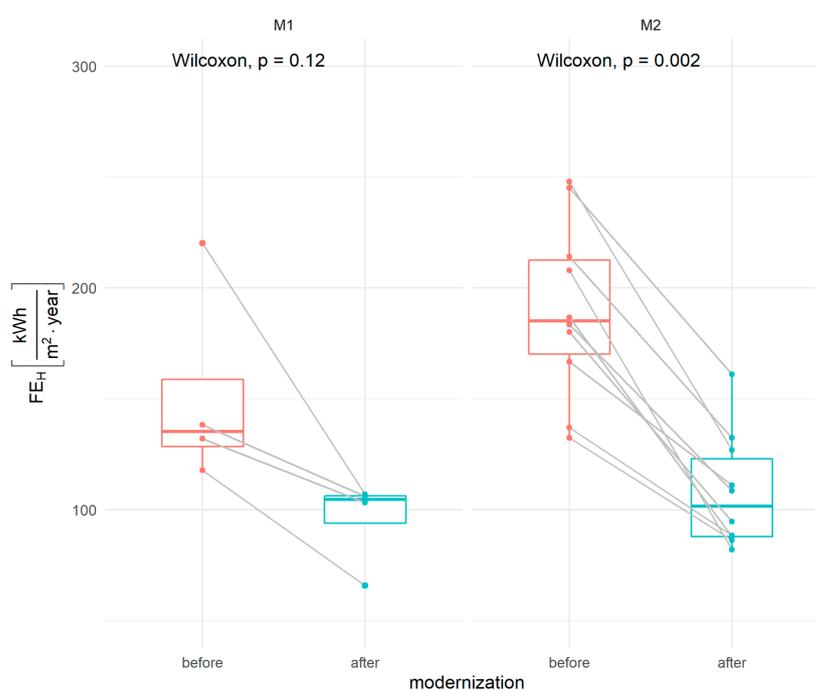
**Figure 2.** The change in  $FE_H$  index value [ $\text{kWh}\cdot\text{m}^{-2}\cdot\text{year}^{-1}$ ].**Table 8.** Average values of the  $FE_H$  [ $\text{kWh}\cdot\text{m}^{-2}\cdot\text{year}^{-1}$ ].
