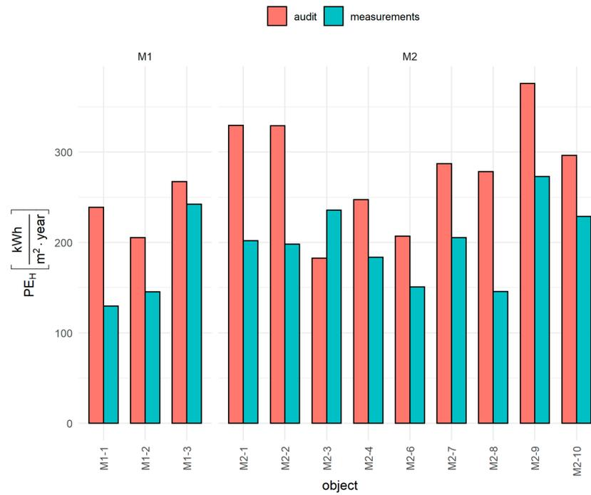
**Figure 4.**  $PE_H$  values obtained from measurements and calculated in the audit before thermal refurbishment.
