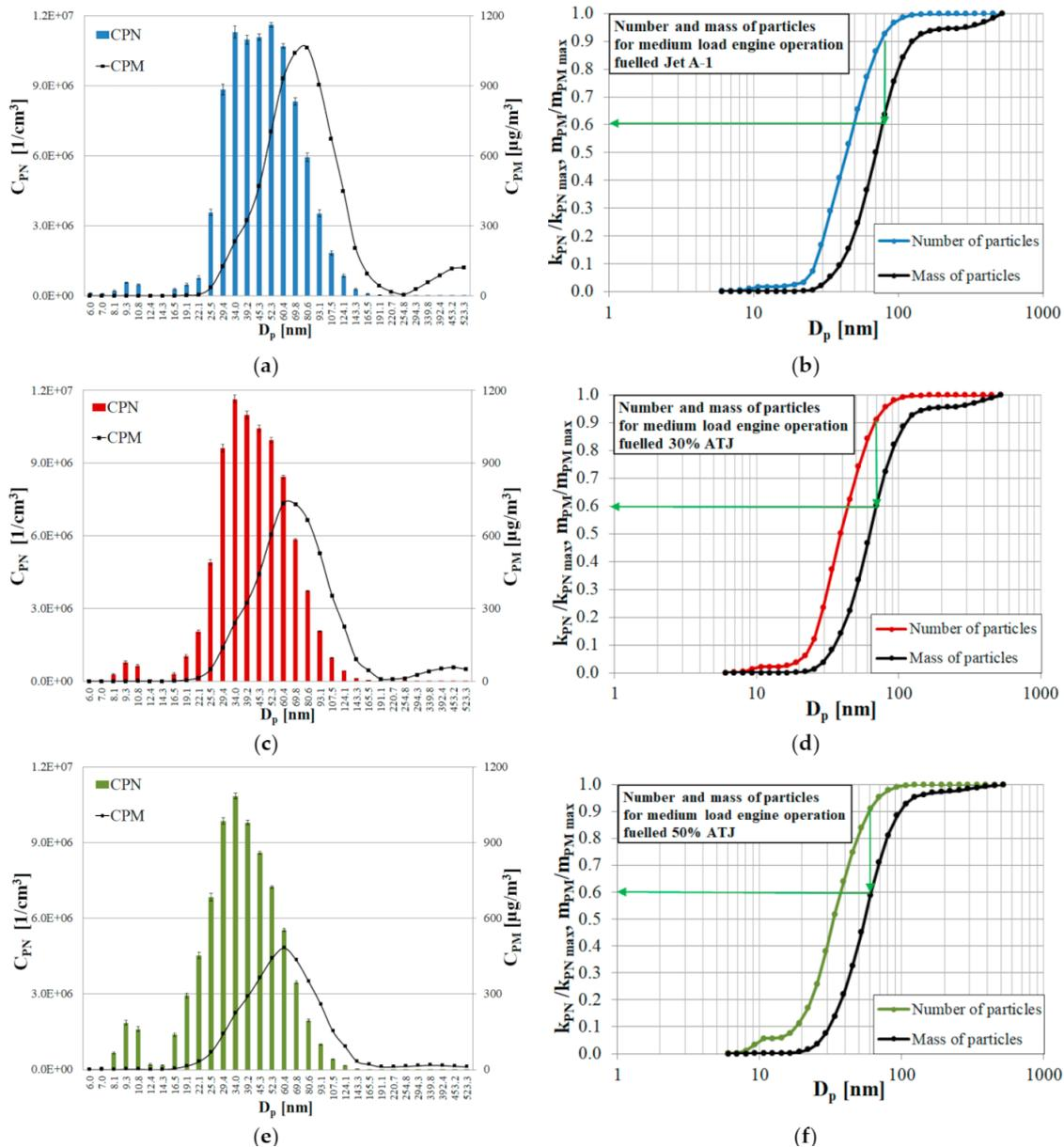
**Figure 6.** Number and mass concentration of particles depending on their diameter (a,c,e) and cumulative values of the relative particles number and relative mass of particulate matter (b,d,f) for medium engine operation load fuelled Jet A-1 (a,b), 30% ATJ (c,d) and 50% ATJ (e,f).
