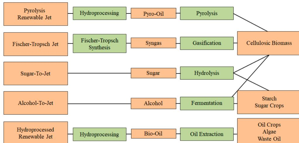
**Figure 1.** Raw materials used for the production of aviation biofuels and the corresponding processing [17].
