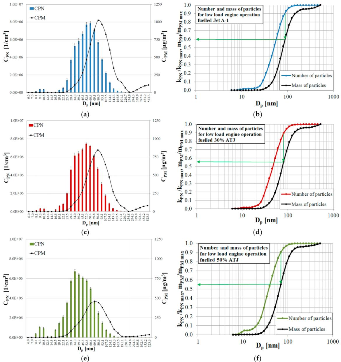
**Figure 5.** Number and mass concentration of particles depending on their diameter (a,c,e) and cumulative values of the relative particles number and relative mass of particulate matter (b,d,f) for low engine operation load fuelled Jet A-1 (a,b), 30% ATJ (c,d) and 50% ATJ (e,f).
