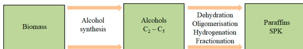
**Figure 2.** Simplified diagram of the ATJ-SPK process [30].
