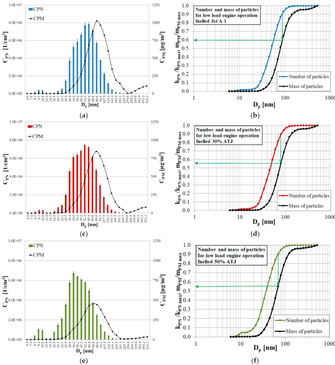
**Figure 5.** Number and mass concentration of particles depending on their diameter (a,c,e) and cumulative values of the relative particles number and relative mass of particulate matter (b,d,f) for low engine operation load fueled Jet A-1 (a,b), 30% ATJ (c,d) and 50% ATJ (e,f).
