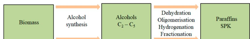
Figure 2. Simplified diagram of the ATJ-SPK process [30].
