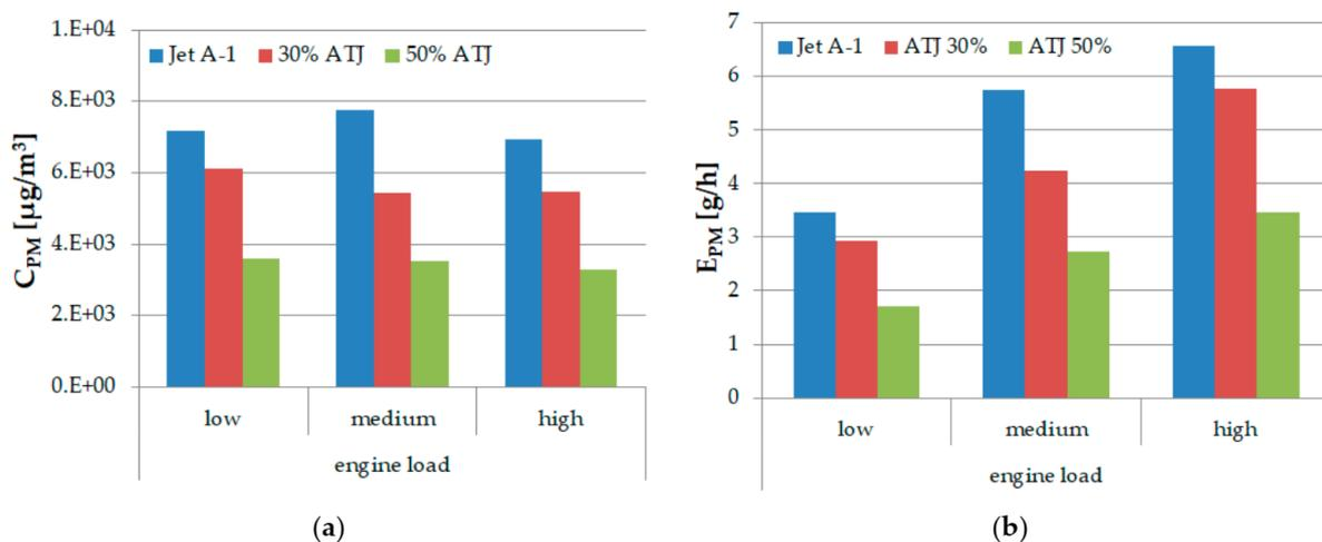
**Figure 9.** Mass concentration  $C_{PM}$  (a) and emission intensity of particulate matter  $E_{PM}$  (b) for tested fuels in three engine operation ranges.
