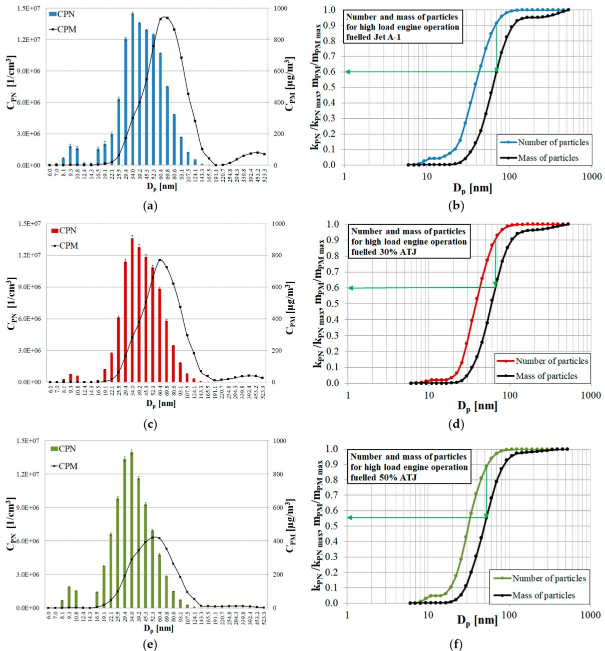
**Figure 7.** Number and mass concentration of particles depending on their diameter (a,c,e) and cumulative values of the relative particles number and relative mass of particulate matter (b,d,f) for high engine operation load fuelled Jet A-1 (a,b), 30% ATJ (c,d) and 50% ATJ (e,f).
