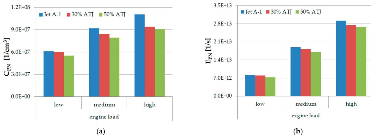
**Figure 8.** The number concentration  $C_{PN}$  (a) and intensity of the particles number emission  $E_{PN}$  (b) for tested fuels in three ranges of engine operation.
