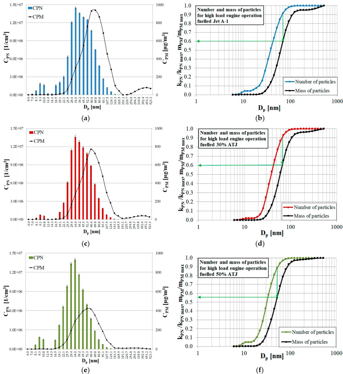
**Figure 7.** Number and mass concentration of particles depending on their diameter (a,c,e) and cumulative values of the relative particles number and relative mass of particulate matter (b,d,f) for high engine operation load fueled Jet A-1 (a,b), 30% ATJ (c,d) and 50% ATJ (e,f).
