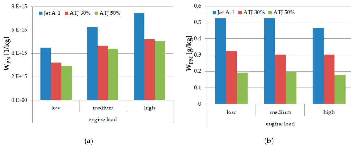
**Figure 10.** Particle number index  $W_{PN}$  (a) and particle mass index  $W_{PM}$  (b) for tested fuels in three engine load ranges.
