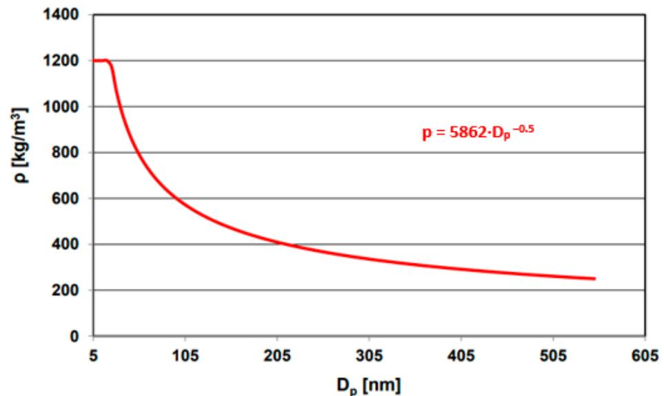
Figure 4. Density of solid particles depending on their diameter [32].
