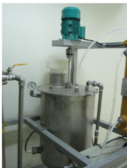
**Figure 5.** The fabricated 70 L reactor for biodiesel production [55].
