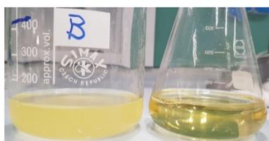
**Figure 7.** A sample of crude biodiesel (left) and purified biodiesel after methanol vacuum distillation (right).
