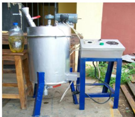
**Figure 4.** The fabricated 20 L unit for biodiesel production [53].
