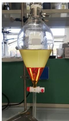
Figure 6. Separation of glycerol phase from biodiesel phase in a lab separating funnel.
