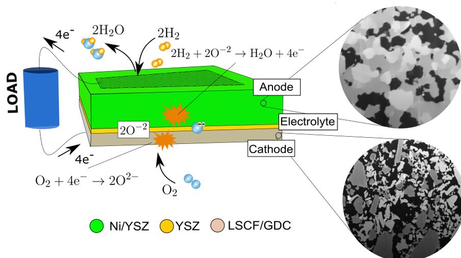
**Figure 1.** Schematic view on solid oxide fuel cell and microstructure of the anode and the cathode.
