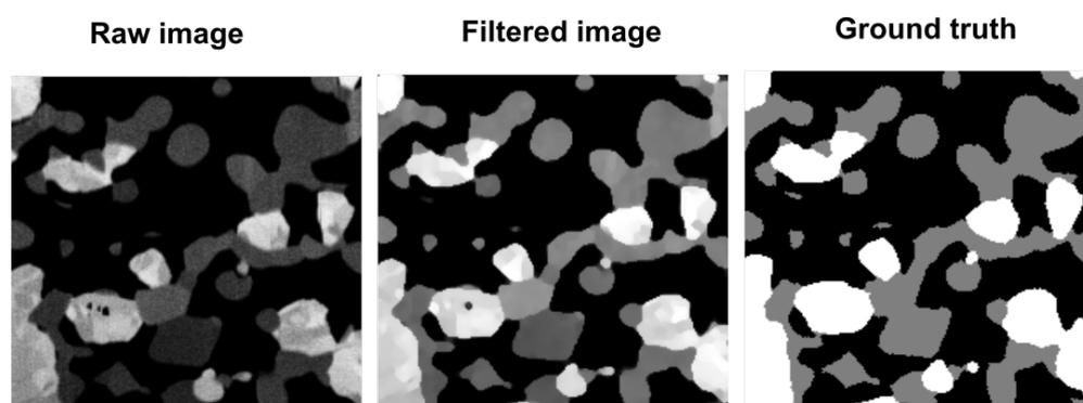
**Figure 2.** Example of filtration performed on a raw FIB-SEM image juxtaposed with an image segmented by the operator.
