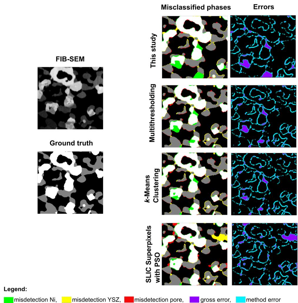
**Figure 4.** Segmentation results of different algorithms, SLIC Superpixels with PSO, *k*-Means Clustering, Multithresholding and proposed SRG with PSO, for the exemplary raw SEM image ( $200 \times 200$  px) with PSO-aided filtering applied. Manually segmented image taken as a ground truth.
