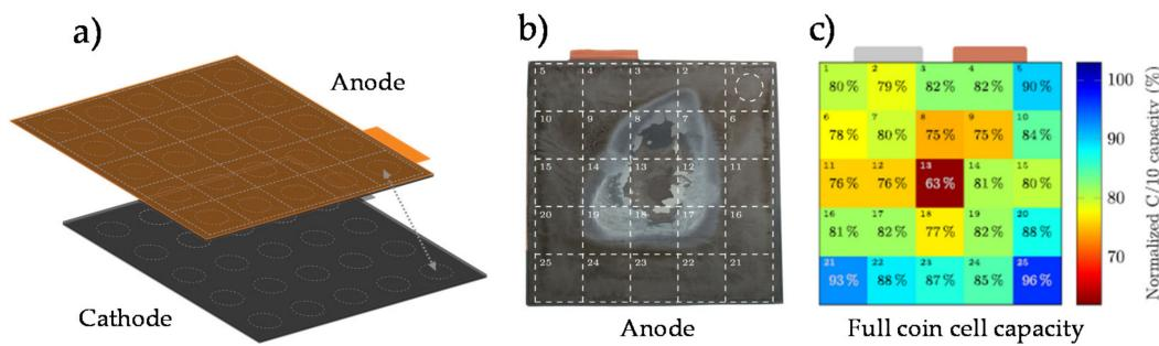
**Figure 8.** Spatially resolved capacity measurement with coin cells: (a) Shows schematic of the location of the samples; (b) Shows one anode sheet and sample locations; (c) Heat map with normalized C/10 capacity with location on the electrodes. Reproduced and modified with permission from [20] Copyright 2020, Elsevier.
