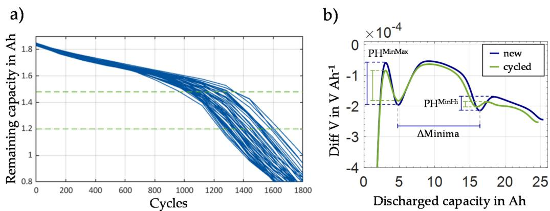
**Figure 10.** Different aging trends and differential voltage analysis: (a) The 48 cells under equal conditions with focus on inherent production caused cell-to-cell variance and capacity degradation over cycles, 80% and 60% of initial capacity are marked with green dashed line. Reproduced from Baumhöfer et al. [61]. (b) Differential voltage analysis on a 25 Ah cell to determine changes in the peak heights to quantify the homogeneity of lithium distribution [126].
