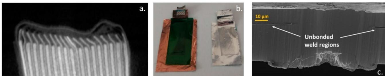
**Figure 4.** Observations of tab deformation and assembling and welding inconsistencies in the Samsung Galaxy Note 7 batteries: (a) X-ray CT scan of electrode deformation in the prismatic cell; (b) missing insulating tape on the cathode tabs; (c) SEM cross-section of an anode tab weld (CC BY Loveridge et al. [81]).
