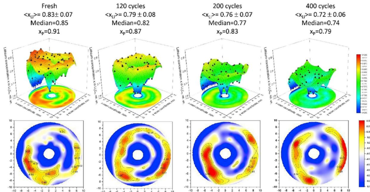
**Figure 7.** Lithium distribution as cross-section determined by differences of reflections of  $\text{LiC}_6$  and  $\text{LiC}_{12}$  phases in graphite with spatially resolved neutron diffraction. Over cycling inhomogeneities enhance. Reproduced with permission from [130] Copyright 2020, Elsevier.
