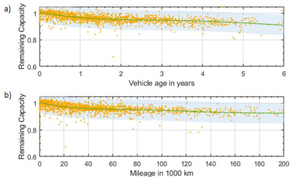
**Figure 12.** Maximal range survey from Tesla Motors, Netherlands forum with reported remaining capacity over: (a) years and (b) mileage from [166]. Each orange dot is one entrance and vehicles can have multiple entries within their life. The trendline is shown in green and 95% confidence interval in light blue.
