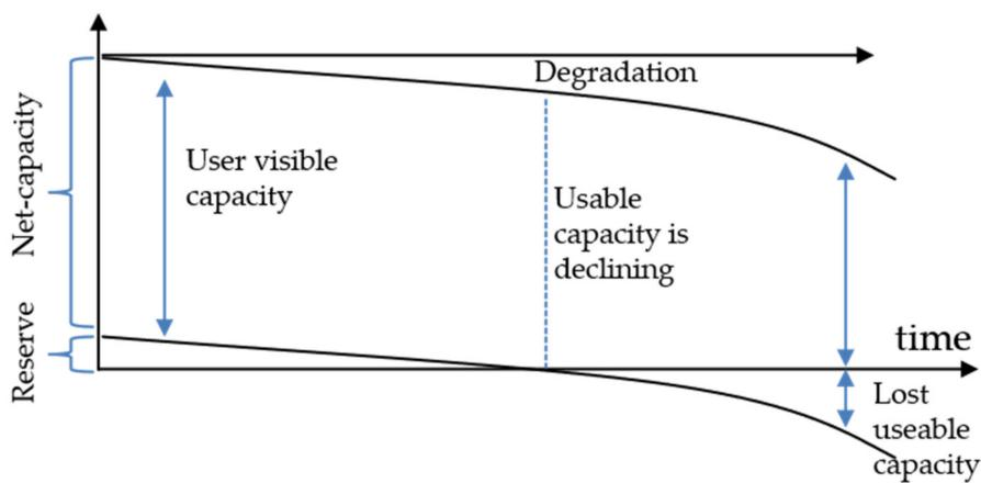
**Figure 13.** User visible capacity from battery management system, reserve is not shown to the user but the state-of-health remains 100% even though degradation already happened.
