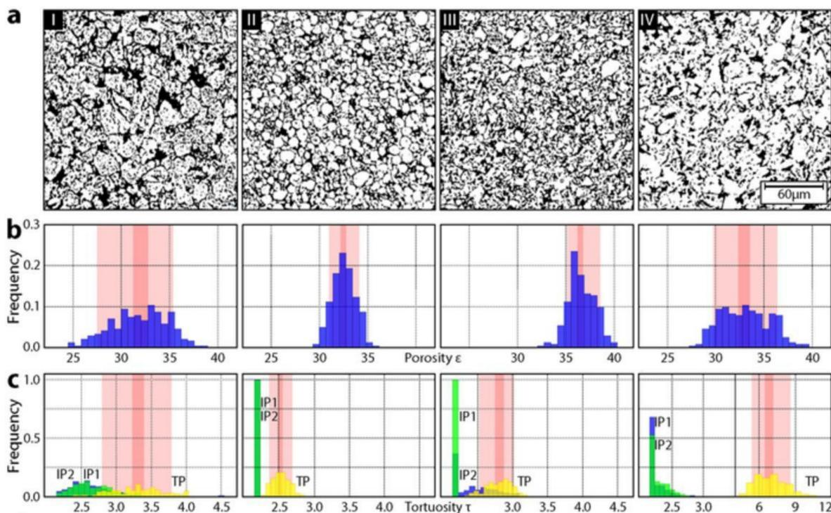
**Figure 2.** Tomogram results of one sample of four different negative electrodes revealing: (a) the types of graphite particles with associated (b) porosity and (c) tortuosity. IP1 and IP2 correspond to two in-plane directions while TP corresponds to the through-plane direction (modified from CC BY Müller et al. [24]).
