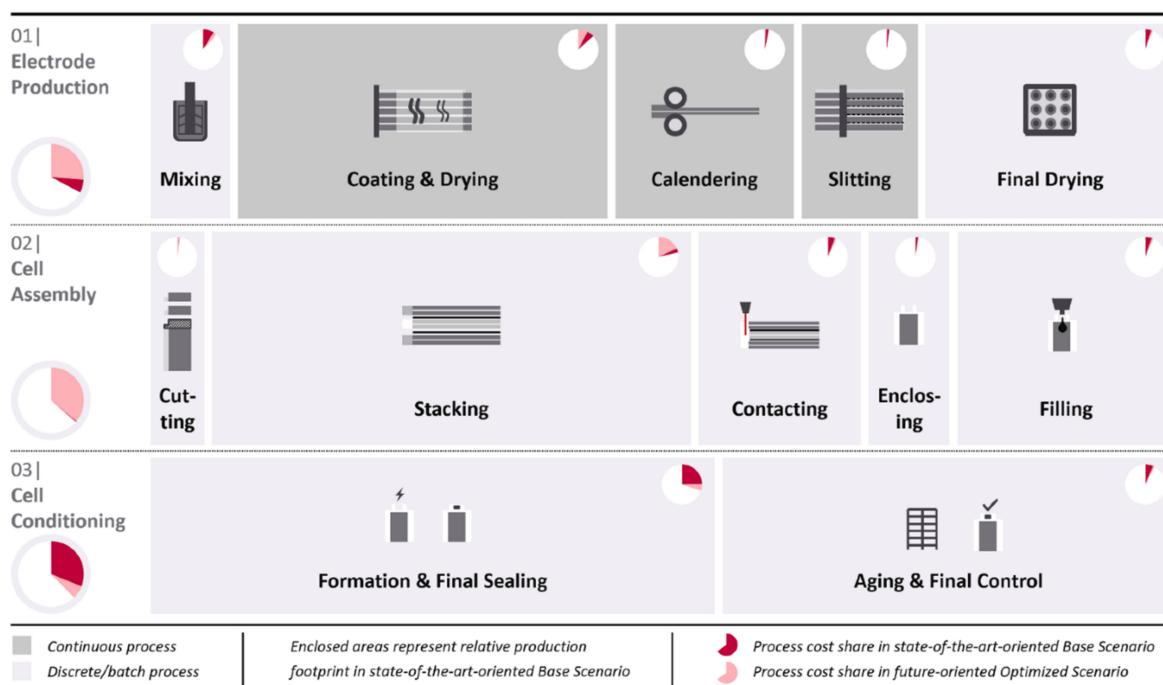
**Figure 3.** Manufacturing process steps of a lithium-ion pouch cells (CC BY Mauler et al. [49]).
