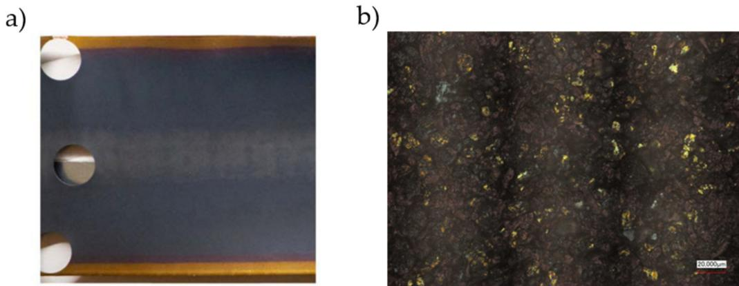
**Figure 9.** Visual inspection of electrodes: (a) Part of the anode of an 18,650 cell with coin cell probes taken in different locations of the cell. The outer part of the electrode shows a different lithiation than the middle part. (Modified from CC BY 4.0 by Spingler et al. [138]); (b) optical microscopy of the outer part of an anode showing individual particles with different lithiation (CC BY 4.0 by Käbitz [142]).
