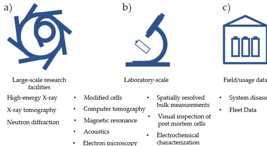
**Figure 5.** Different scales and complexity for ctcV and inhomogeneities measurements: (a) Large scale research facilities; (b) Laboratory-scale; (c) Field usage data.
