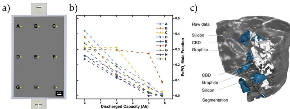
**Figure 6.** 3D reconstruction of electrodes: (a) Location of bulk measurement points, and (b) spatial inhomogeneity during discharge in LFP pouch cell. Reproduced with permission from [59] Copyright 2015, Elsevier. (c) The 3D-reconstruction of tomographic raw data and segmentation of silicon-graphite anode from a transmission X-ray tomographic microscope. Scale bar 15  $\mu\text{m}$ . (CC BY 4.0 Müller et al. [124]).
