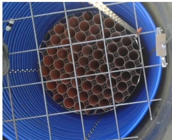
**Figure 3.** Skeletal bed situated in the fermenter, secured with a grid; between the bed and the wall of the fermentor there is a coil-view (photo by Grzegorz Wałowski).
