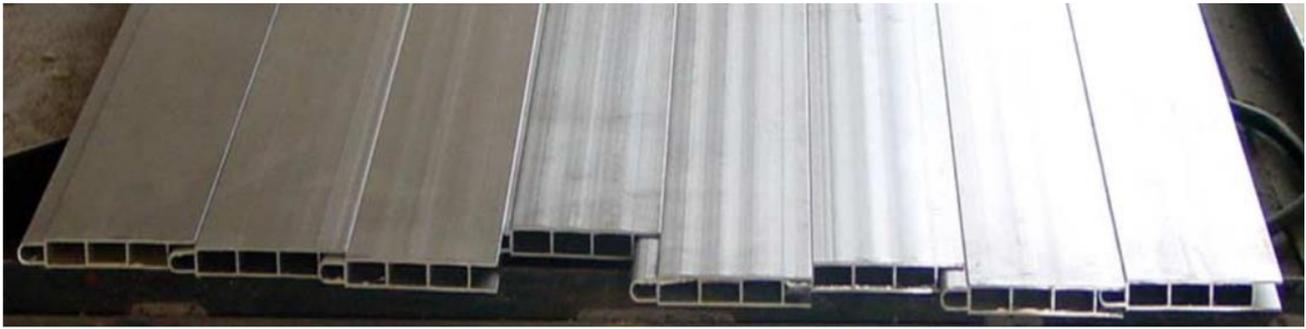
**Figure 8.** Assembly of aluminium finned flow channels (reprinted from [75], with permission from publisher).
