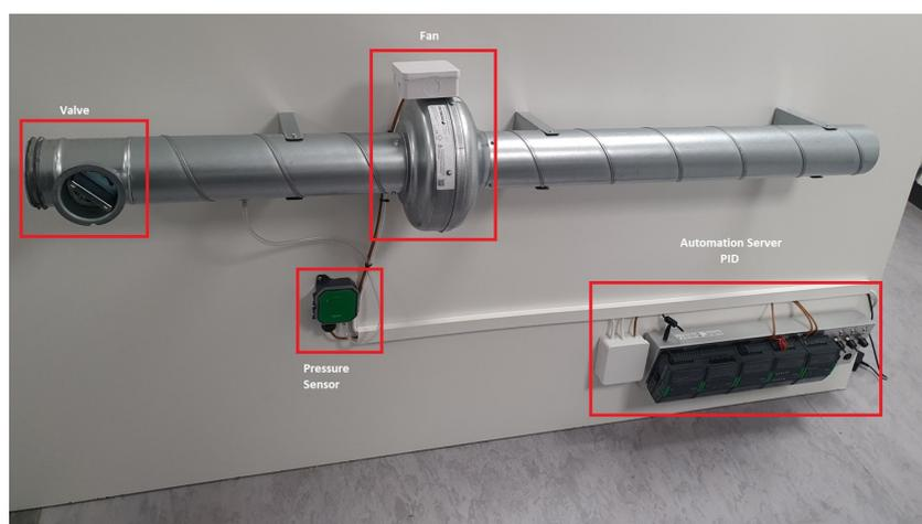
**Figure 8.** Overview of the fan testbed with its components.
