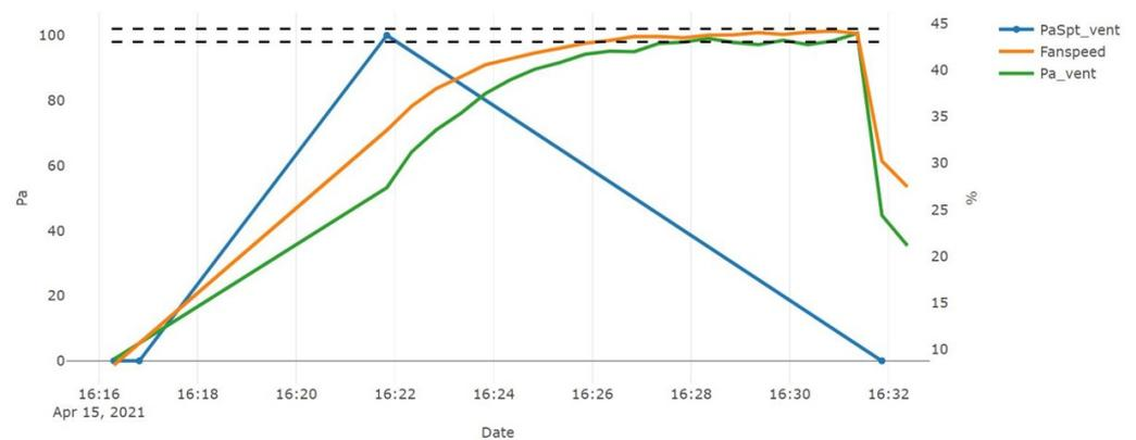
Figure 13. Time step response of the ventilation setup: stable condition.
