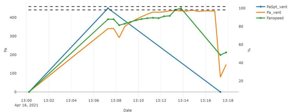
Figure 15. Time step response of the ventilation setup: unstable condition.
