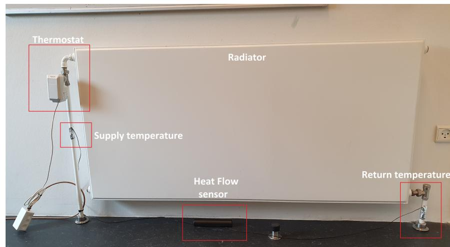
Figure 7. Heating testbed with its components.
