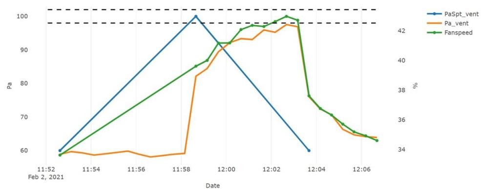
Figure 14. Time step response of the ventilation setup: short stability.
