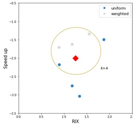
**Figure 2.** Illustration of the  $k$ -NN classifier method to predict the type of regression  $\hat{c}$  (uniform or inverse-distance weighting), used by Algorithm 3. Red diamond: target site. The circles group the  $k = 4$  nearest neighbors in the 2-dimensional space created by the features  $speedup$  and  $RIX$ . The same idea holds for predicting the number of neighbors  $\hat{k}$ .
