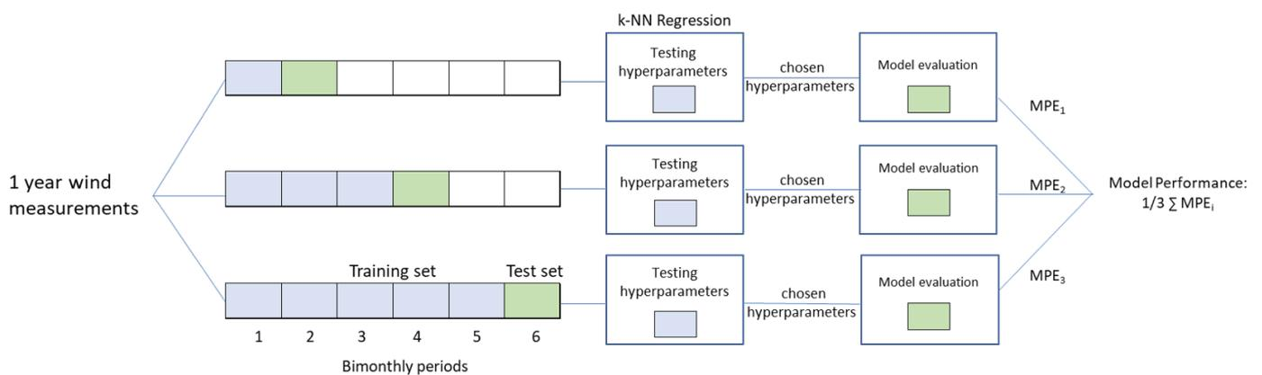
**Figure 3.** Illustration of the nested hyperparameter estimation and cross-validation approach.
