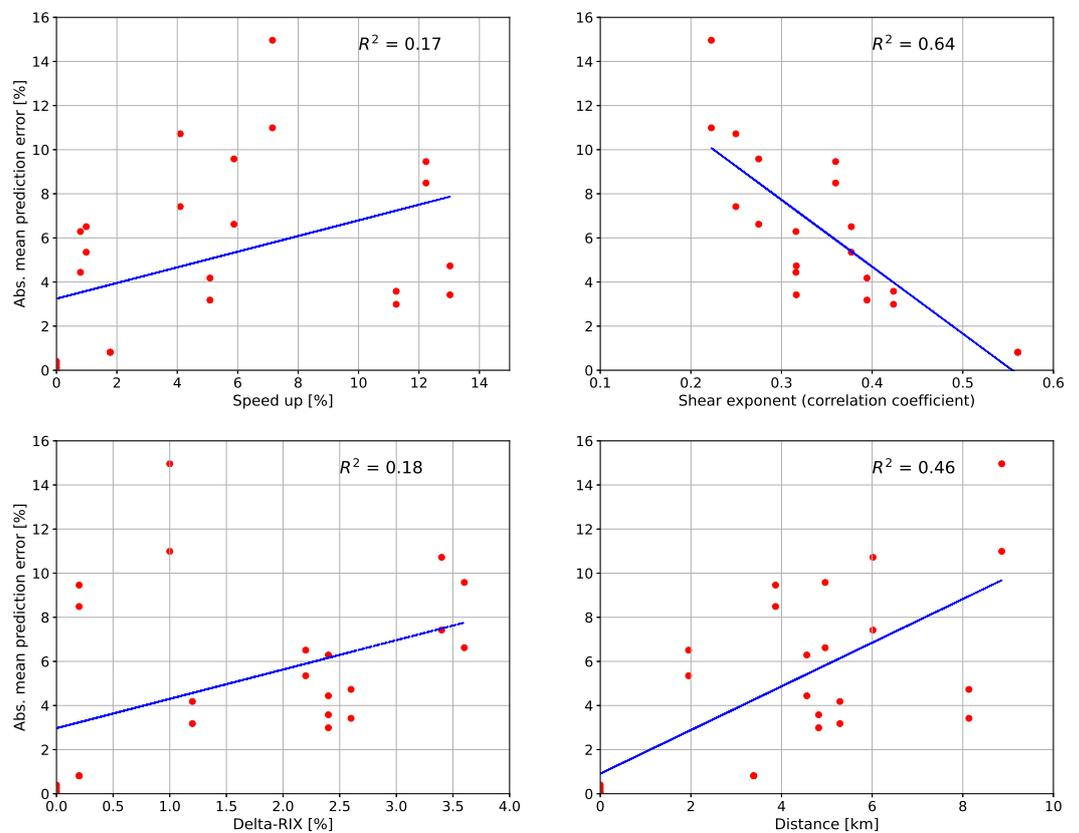
**Figure 4.** Mean absolute modeling error for WASP-predicted wind speed vs. features selected for the  $k$ -NN study. The dots correspond to the cross-validation between each pair of sites. The blue line represents the linear regression of the errors as a function of presented features.
