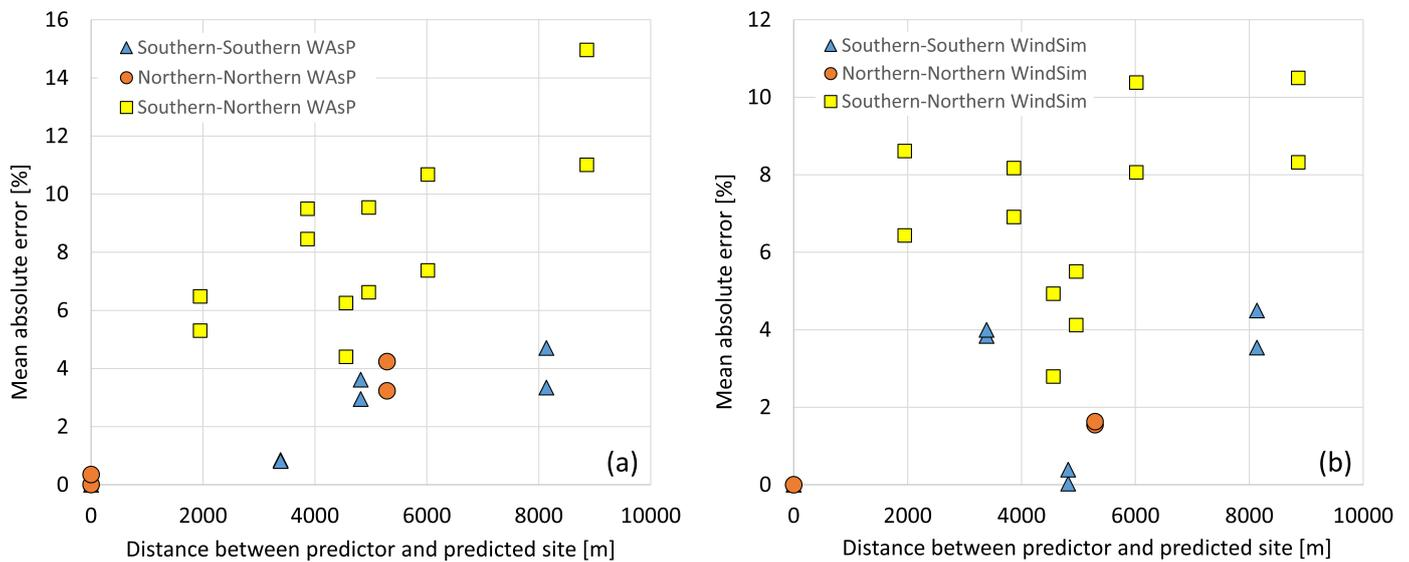
**Figure 7.** Absolute mean prediction error of the cross-validations as a function of distance and zone for the results using (a) WASP; and (b) WindSim.
