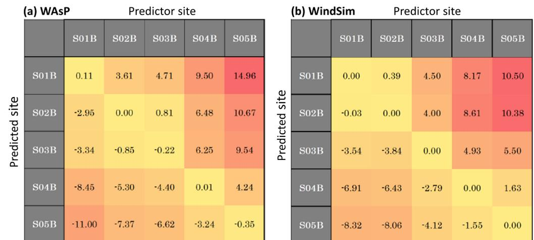
**Figure 6.** Cross-validation errors for the prediction of the average wind speed in % obtained with WAsP (a) and WindSim (b). Light orange colors: small errors; reddish colors: large errors.
