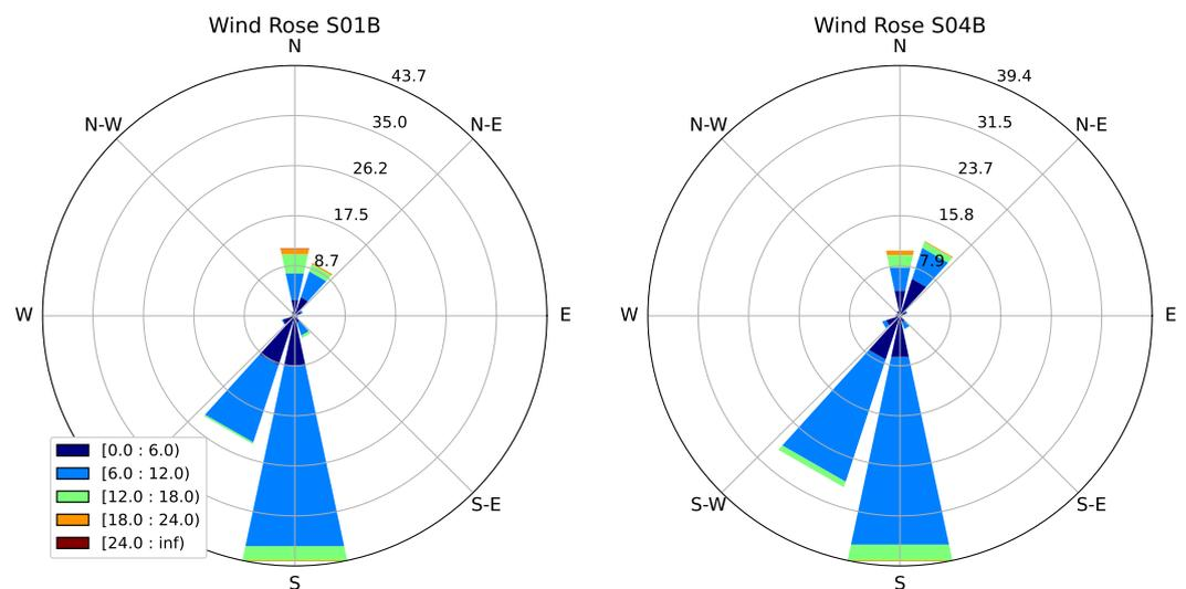
**Figure 5.** Wind rose observed at sites S01B and S04B from June 2016 to June 2017.
