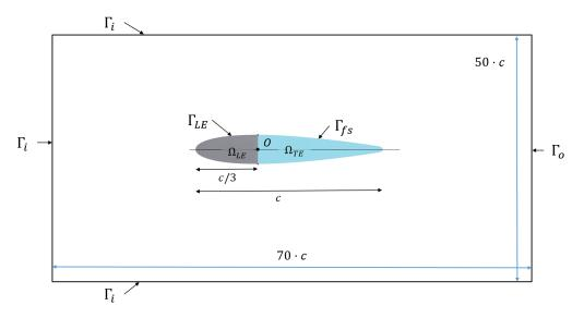
**Figure 2.** Partly deformable hydrofoil geometry, fluid, and solid domains boundaries:  $\Omega_{LE}$  (gray) is non deformable and  $\Omega_{TE}$  (cyan) is deformable.
