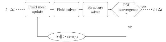
Figure 3. FSI implicit coupling scheme.
