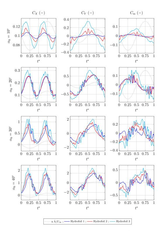
**Figure 8.** Hydrodynamic coefficients  $C_Y$ ,  $C_M$ , and  $C_X$  and hydrofoil vertical velocity  $\dot{h}/U_{\infty}$  versus time, for  $\alpha_0 = 10^\circ$ ,  $20^\circ$ ,  $30^\circ$ , and  $40^\circ$  and  $f^* = 0.025$ ,  $\Delta h = 0.8$  m and for the three materials.
