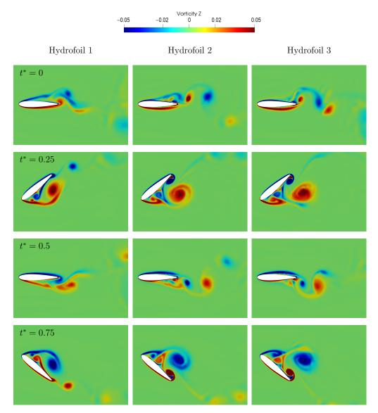
**Figure 7.** Instantaneous vorticity fields  $\omega_z$  around the oscillating hydrofoil for the hydrofoils 1, 2, and 3,  $\alpha_0 = 40^\circ$ ,  $f^* = 0.025$ ,  $\Delta h = 0.8$  m, and  $t^* = 0$ , 0.25, 0.5, 0.75.
