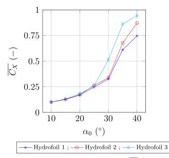
**Figure 9.** Mean hydrodynamic coefficient  $\overline{C_X}$  versus pitching amplitude  $\alpha_0$  for  $f^* = 0.025$ ,  $\Delta h = 0.8$  m, and for the three materials.
