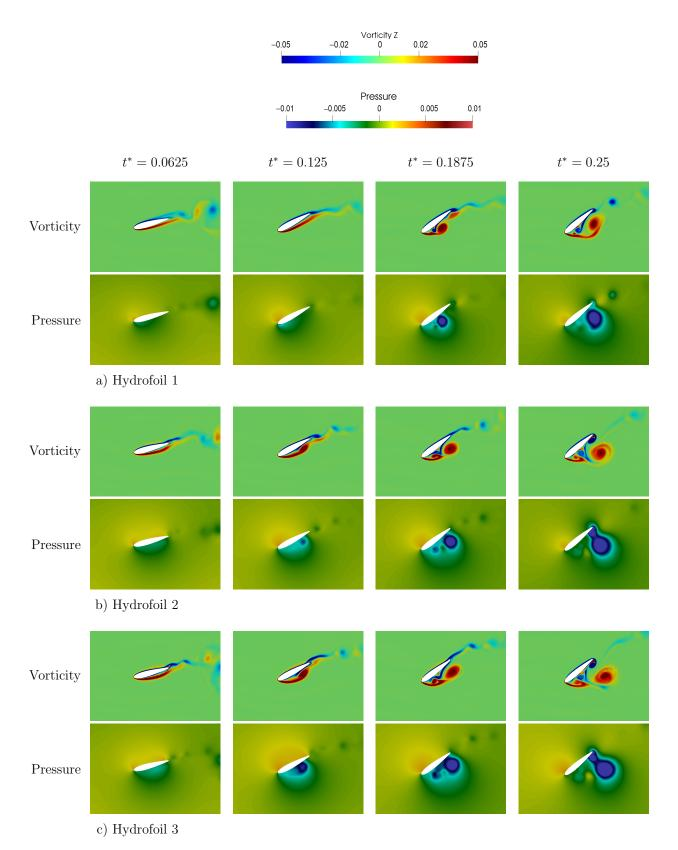
**Figure 11.** Vorticity and pressure fields around the oscillating hydrofoils (1–3) for  $\alpha_0 = 40^\circ$ ,  $f^* = 0.025$ , and  $\Delta h = 0.8$  m, at times  $t^* = 0.0625$ , 0.125, 0.1875, and 0.25.
