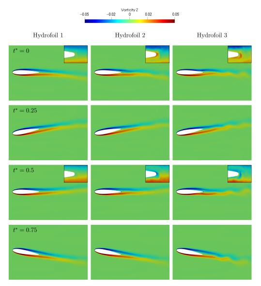
**Figure 5.** Instantaneous vorticity fields  $\omega_z$  around the oscillating hydrofoil for the hydrofoils 1, 2, and 3,  $\alpha_0 = 10^\circ$ ,  $f^* = 0.025$ ,  $\Delta h = 0.8$  m, and  $t^* = 0$ , 0.25, 0.5, 0.75.
