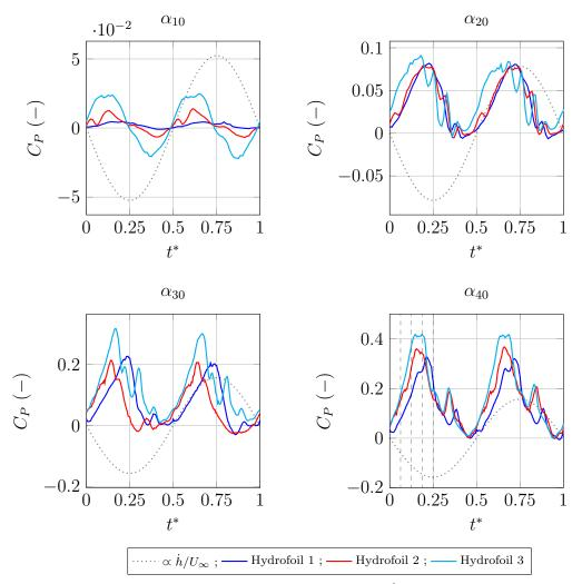
**Figure 10.** Power coefficient  $C_P$  and hydrofoil vertical velocity  $\dot{h}/U_{\infty}$  versus time, for  $\alpha_{10}$  to  $\alpha_{40}$ ,  $f^* = 0.025$ ,  $\Delta h = 0.8$  m, and for three materials.
