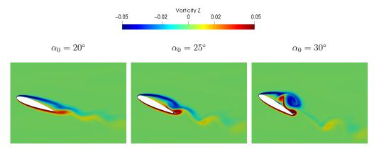
**Figure 6.** Instantaneous vorticity fields  $\omega_z$  around the oscillating hydrofoil 2,  $\alpha_0 = 20$ , 25 and 30°,  $f^* = 0.025$ ,  $\Delta h = 0.8$  m, and  $t^* = 0.75$ .
