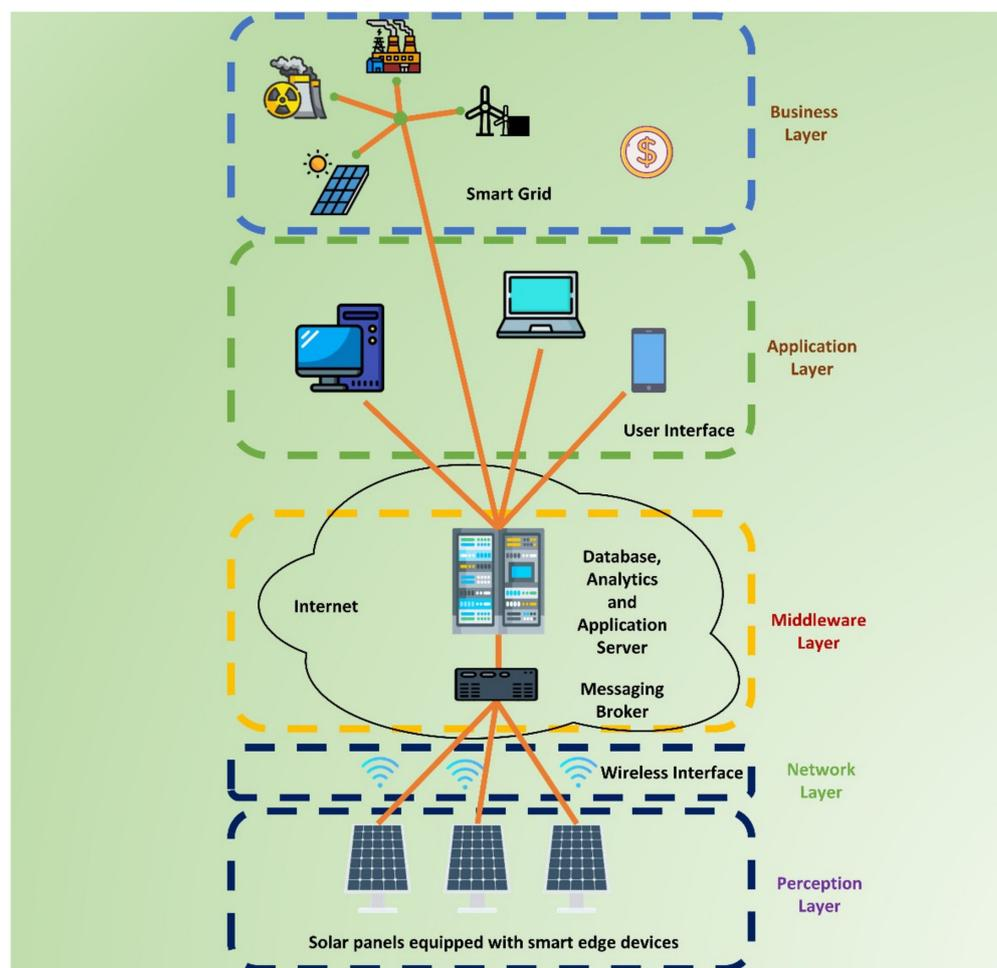
**Figure 6.** IoT-based PV power monitoring and control architecture.
