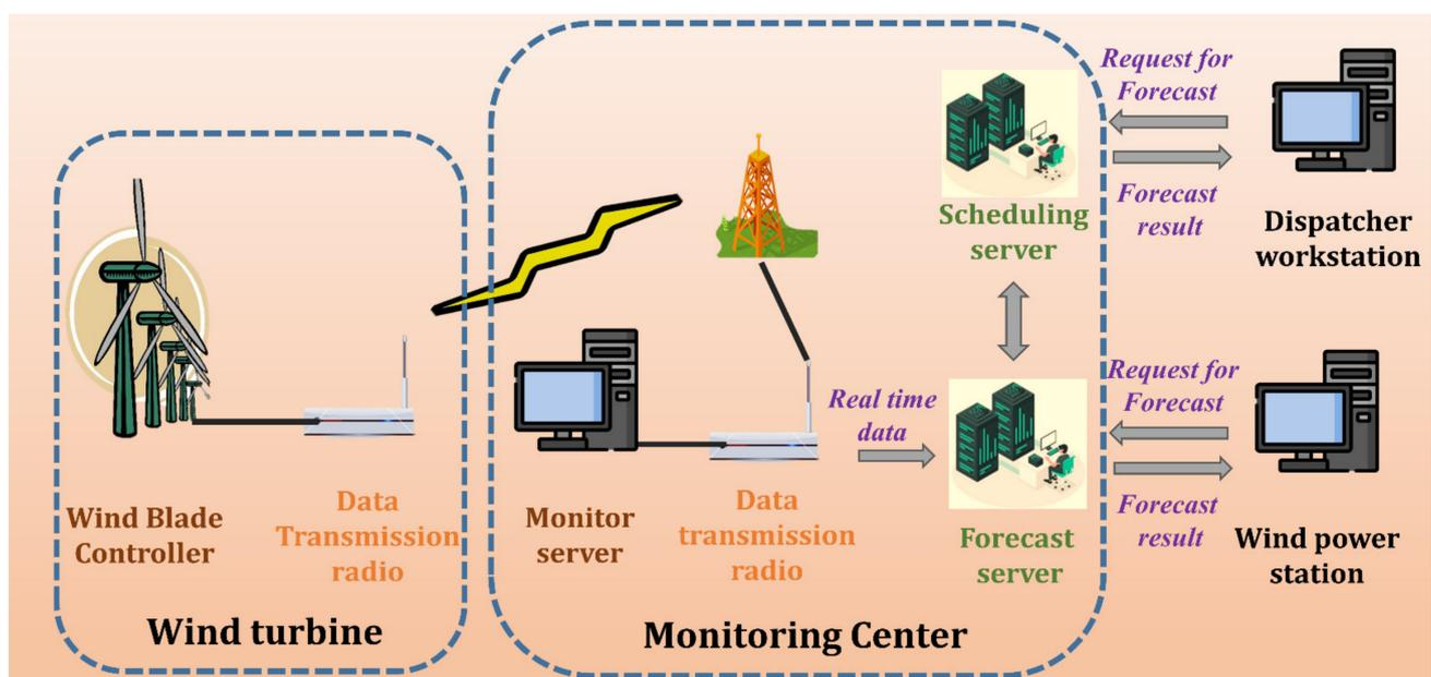
Figure 5. IoT-based wind power monitoring architecture.
