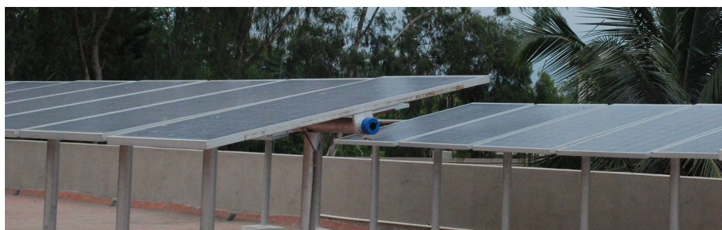
Figure 8. Array of several 300 W PV modules under test in a rooftop setting.
