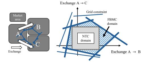
Figure 4. Comparison of the exchange domain between NTC and FBMC.
