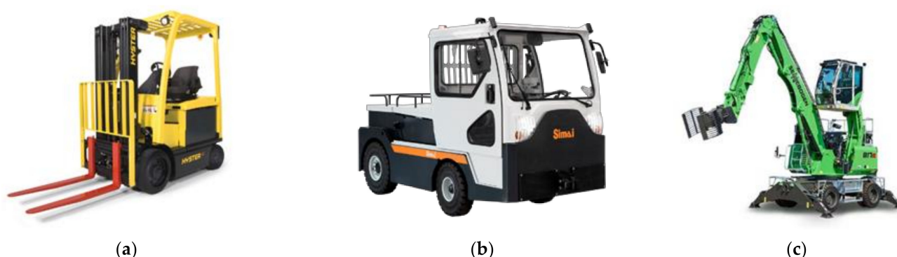
Figure 11. Goods transportation and material handling vehicles. (a) Hyster-Yale forklift. (b) Simai towing tractor. (c) Sennebogen material handler. [89–91].
