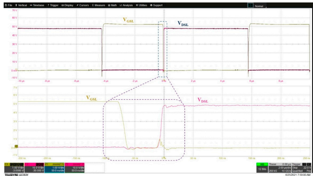
Figure 25. Experimental waveforms of the gate-source voltage of the lower device of inverter leg (phase a) under the rise of the inverter leg node voltage (lower device-drain-source voltage). The dv/dt effect acts a gate voltage spike under the GaN threshold voltage ( V_{GTH} ) V_{DSL}=10 V/div, V_{GSL}=1 V/div, t_{main}=2 \mu s, t_{zoom}=50 ns/div.
