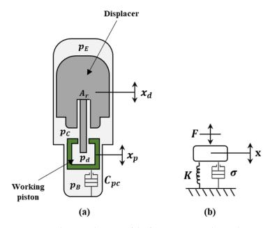
**Figure 6.** A schematic drawing of the forces acting on the working piston and the displacer (**a**) and the mass-spring-damper system approximation (**b**).
