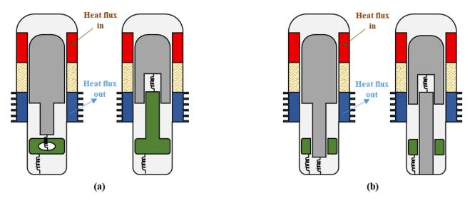
**Figure 3.** Two common models of single-acting working piston-displacer in tandem FPSE: (**a**) displacer sprung to working piston; (**b**) displacer piston sprung to ground.
