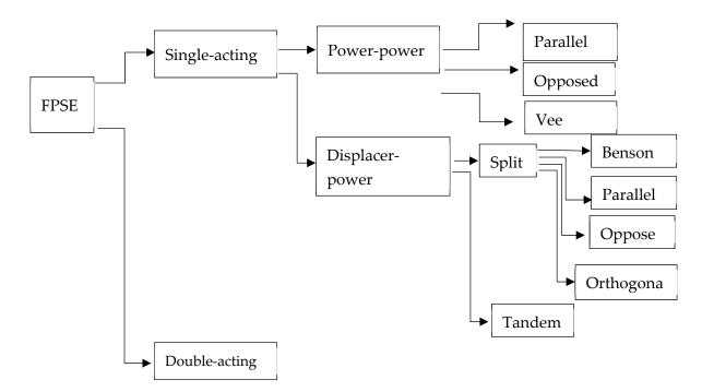
Figure 2. Classification of single-acting and double-acting FPSEs.
