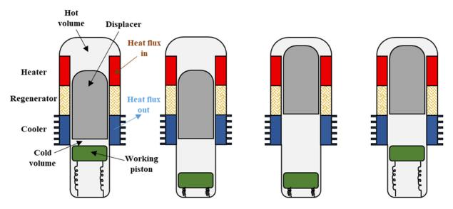
Figure 1. Operation mode of a FPSE [26].
