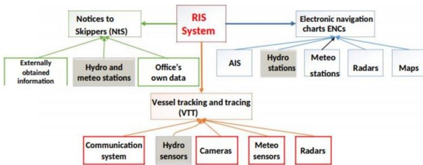
**Figure 2.** RIS system diagram. Source: Own elaboration
