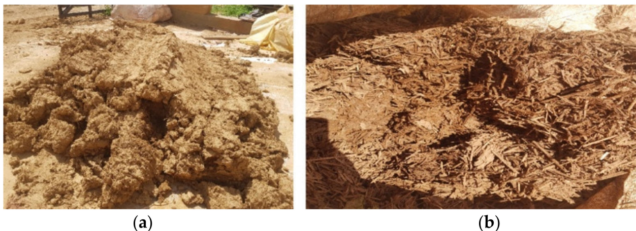
Figure 6. Photos of the studied cob mixes: (a) structural cob material, (b) insulation cob material.
