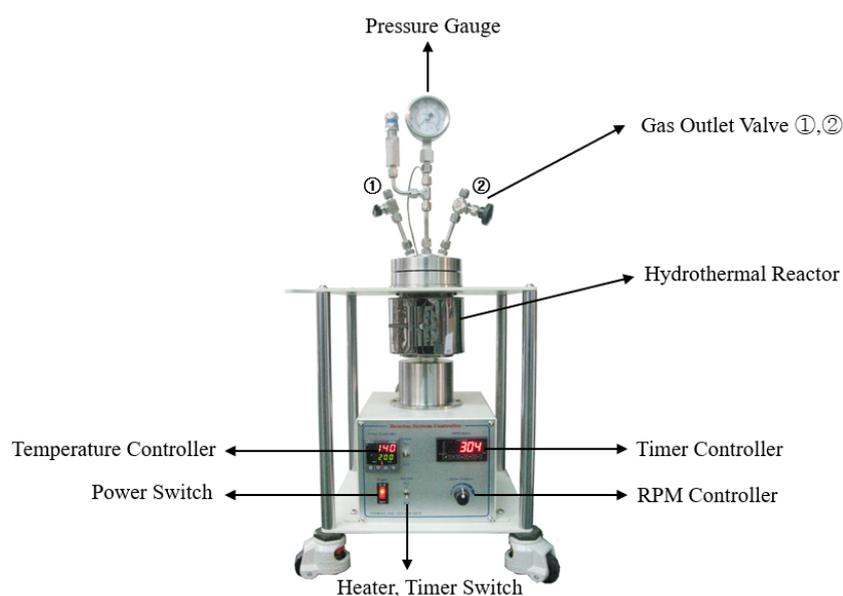
**Figure 2.** The hydrothermal reactor used in this study.
