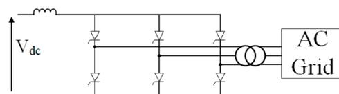
Figure 10. Line-commutated converter.
