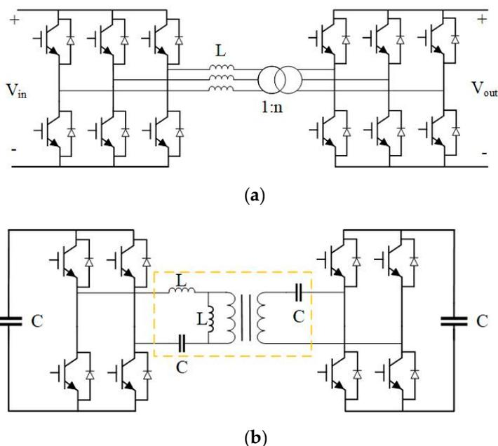
Figure 15. (a) Dual active bridge (DAB), (b) DAB-resonant converter.
