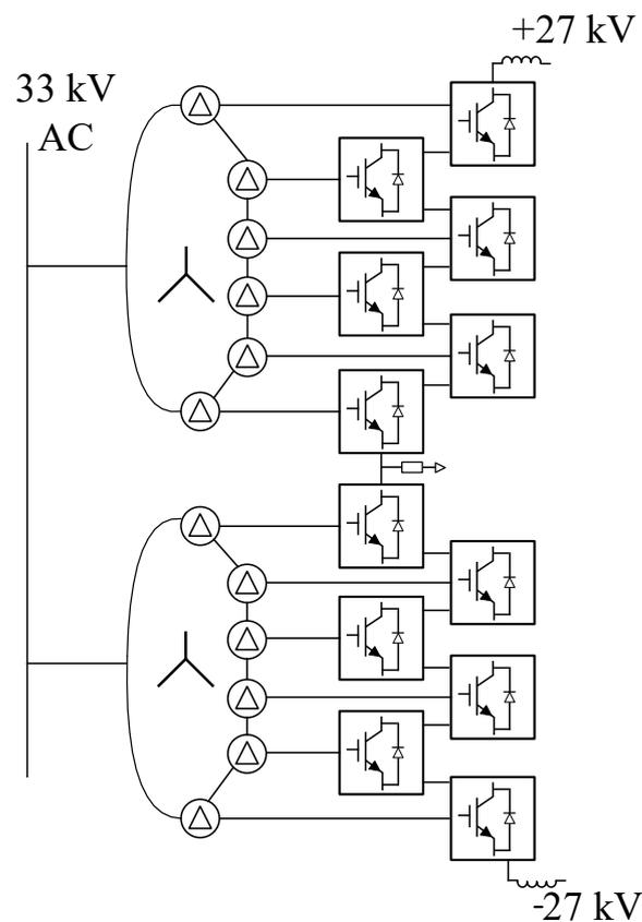
**Figure 13.** Converter station configuration of Angle-DC Project.
