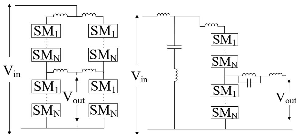
**Figure 17.** Push–pull and tuned filter MMDC.
