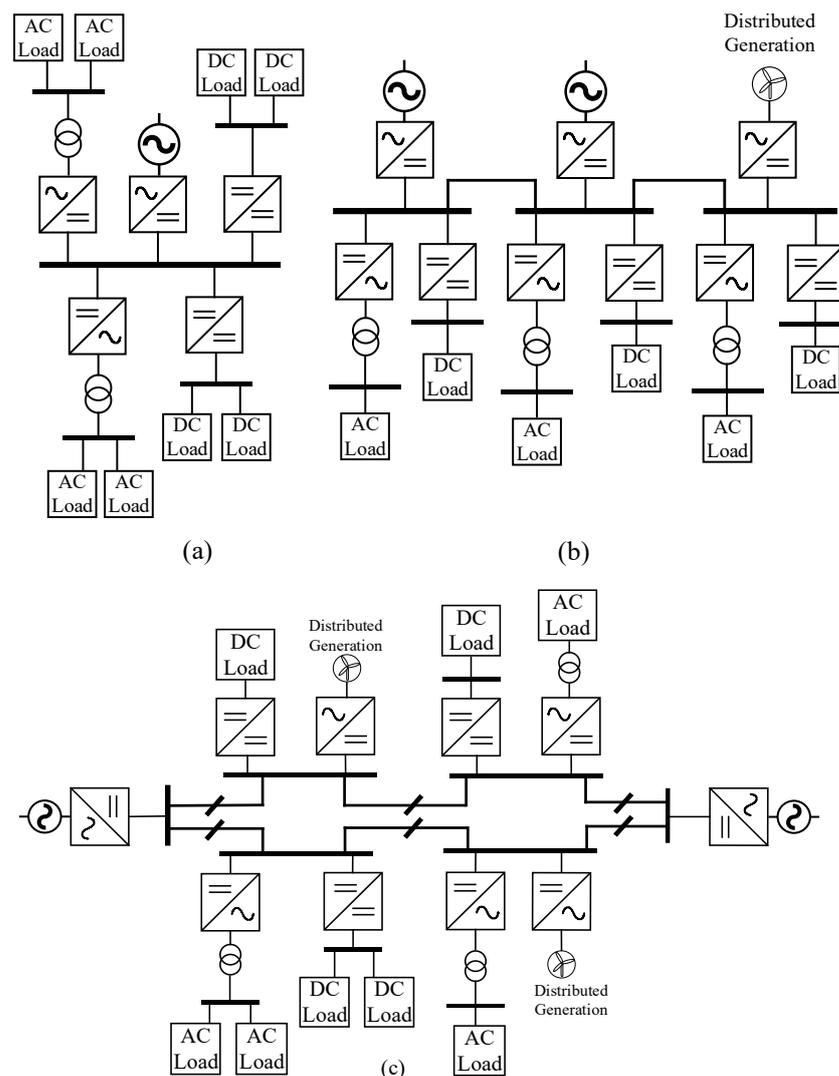
Figure 8. Network topologies: (a) radial, (b) hand-in-hand multiterminal, and (c) ring.
