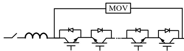
Figure 18. Solid-state DC circuit breaker.
