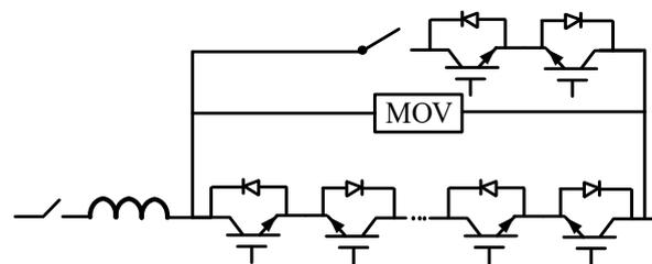
Figure 19. Hybrid DC circuit breaker.
