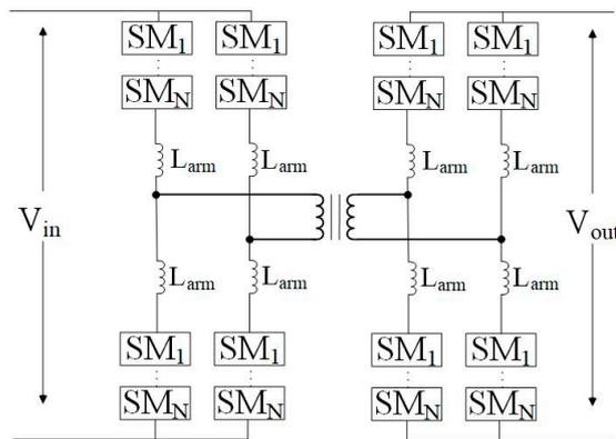
**Figure 16.** Dual active bridge modular multilevel converter.
