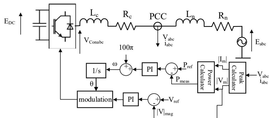
**Figure 21.** Virtual synchronous machine general control.
