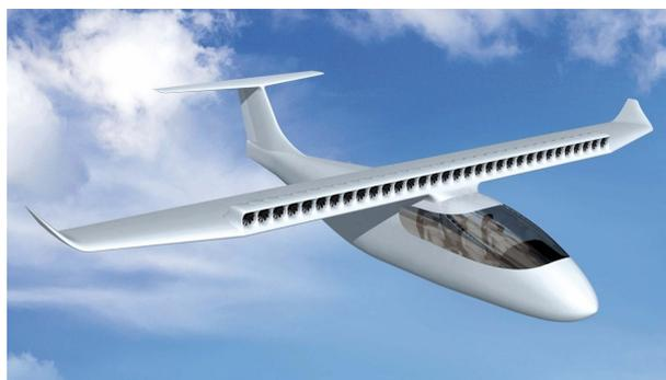
**Figure 8.** Distributed electric propulsion creating higher bypass ratio and lift wing [26].
