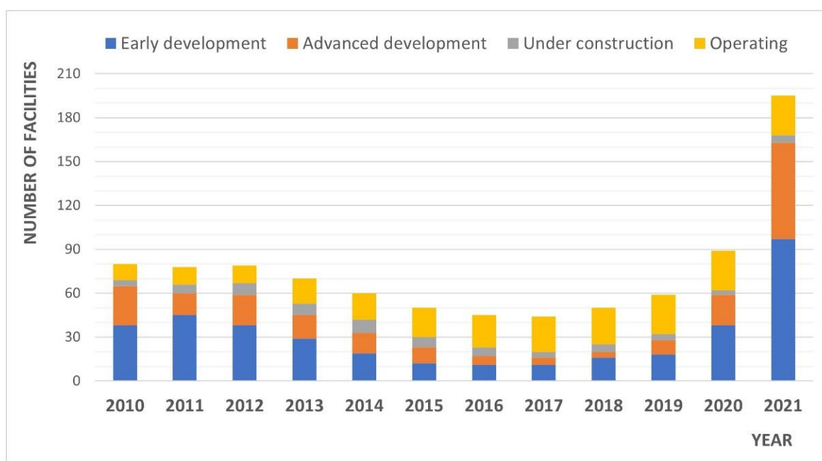
Figure 10. Commercial CCS facilities operating and under development [6,64–67].
