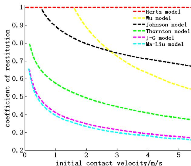
Figure 2. Comparison of the coefficient of restitution models.
