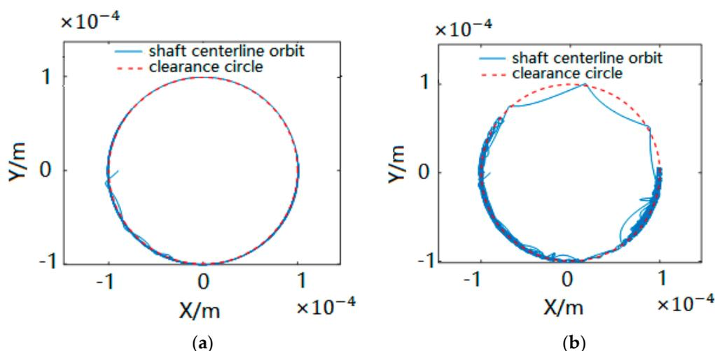
**Figure 12.** Shaft centerline orbit: (a) the constant coefficient of restitution model, (b) the new coefficient of restitution model.
