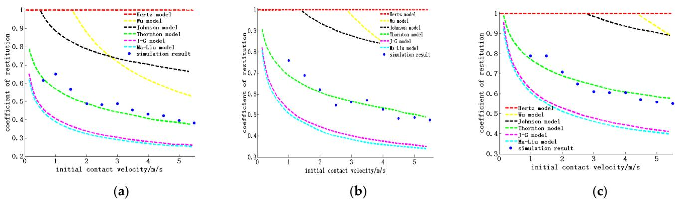
**Figure 4.** Influence of the yield strength of the ball on the coefficient of restitution: (a) yield strength of 400 MPa, (b) yield strength of 600 MPa, (c) yield strength of 800 MPa.
