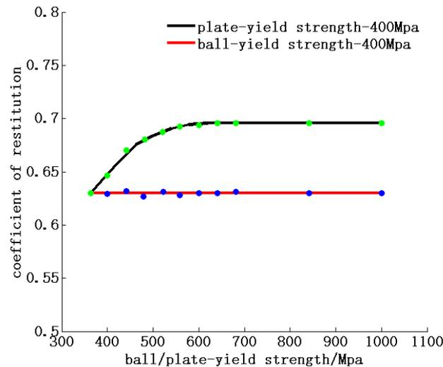
Figure 6. Influence of different yield strength ratios on the coefficient of restitution.
