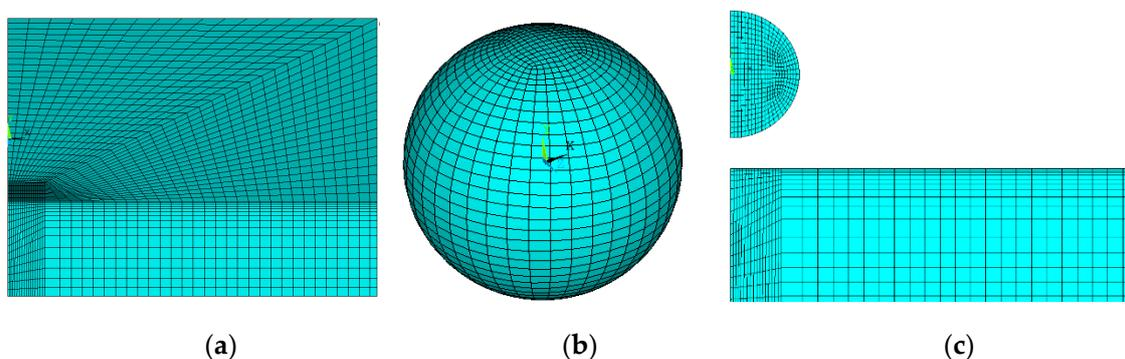
**Figure 3.** Mesh division during ball–plate collision: (a) matrix meshing, (b) ball meshing, (c) three-dimensional model of ball–plate collision.
