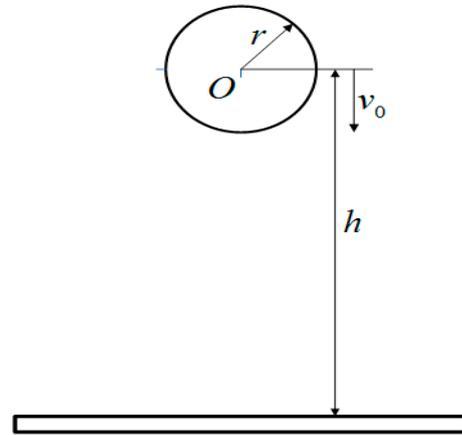
Figure 1. Classic ball–plate collision model.
