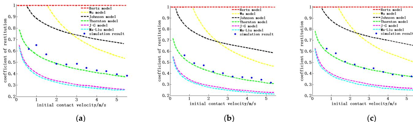
**Figure 5.** Influence of different materials on the coefficient of restitution: (a) collision of steel balls and rigid plates, (b) collision of aluminum balls and rigid plates, (c) collision of copper balls and rigid plates.
