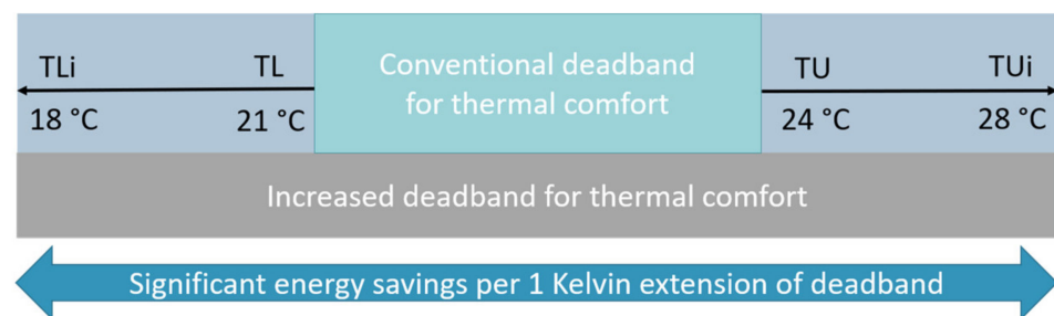
Figure 5. Increased deadband compared to a conventional deadband: the deadband is marked with the lower setpoint temperature TL (heating setpoint) and the upper setpoint temperature TU (cooling setpoint); TLi and TUi mark the initial setpoints for the adaptive controller.
