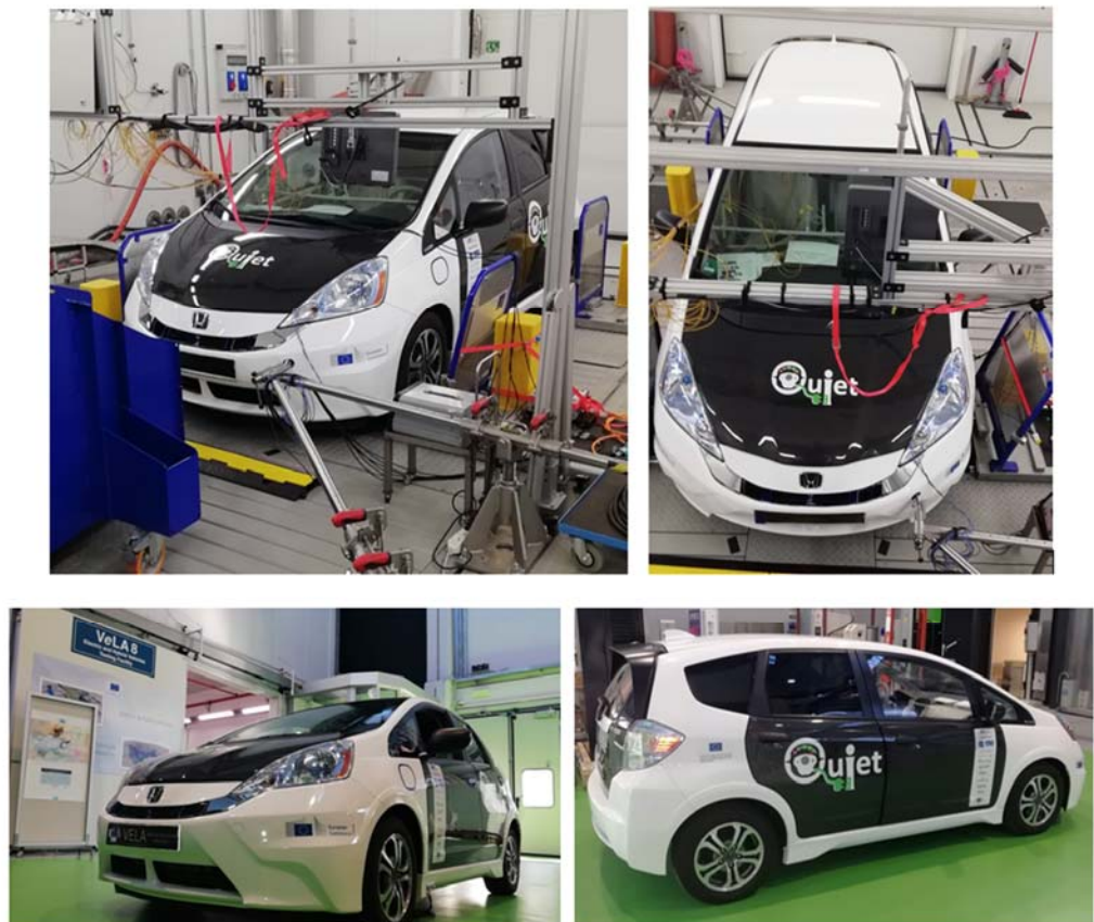
Figure 3. QUIET demonstrator tested at the JRC Ispra VeLA 8 facility [18,23,24]. Image © European Union, 2021.
