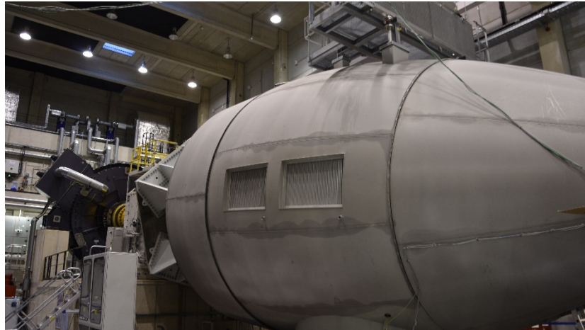
Figure 1. State-of-the-art multi-megawatt nacelle test bench at the Center for Wind Power Drives, RWTH Aachen University, with an ENERCON E-115 E2 mounted.
