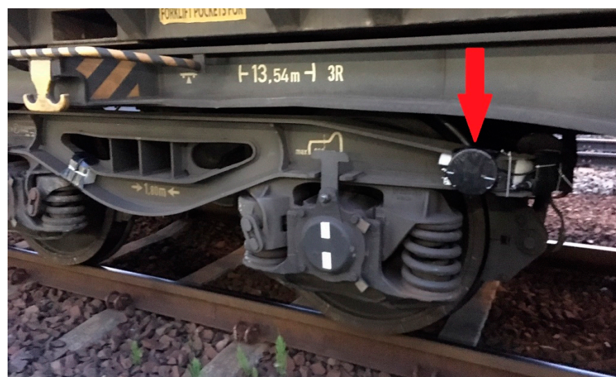
Figure 13. The converter is mounted on the 25TN bogie frame.
