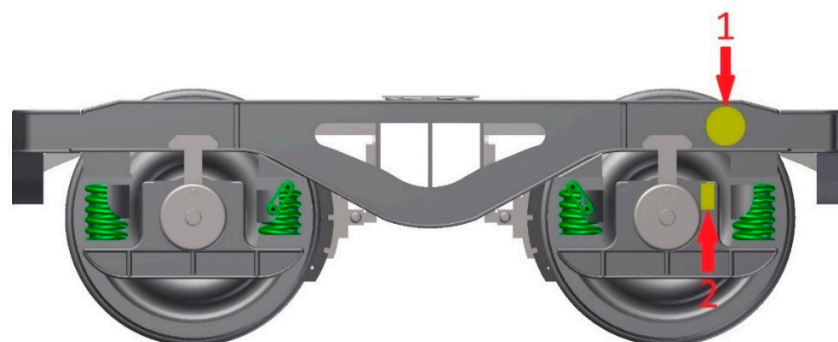
Figure 2. The place of installation of the measuring sensor and harvester on the freight wagon cart.
