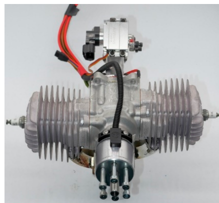
Figure 3. The two-stroke, SI aviation piston engine.
