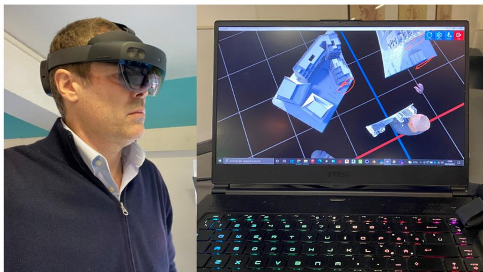
**Figure 7.** MR collaborative environment with MS HoloLens 2.
