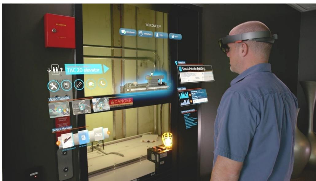
**Figure 8.** ThyssenKrupp MR solution for elevator maintenance.
