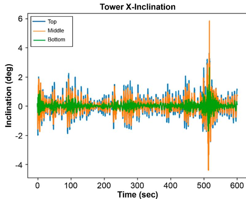
Figure 24. Inclination of wind turbine tower in Case 3.
