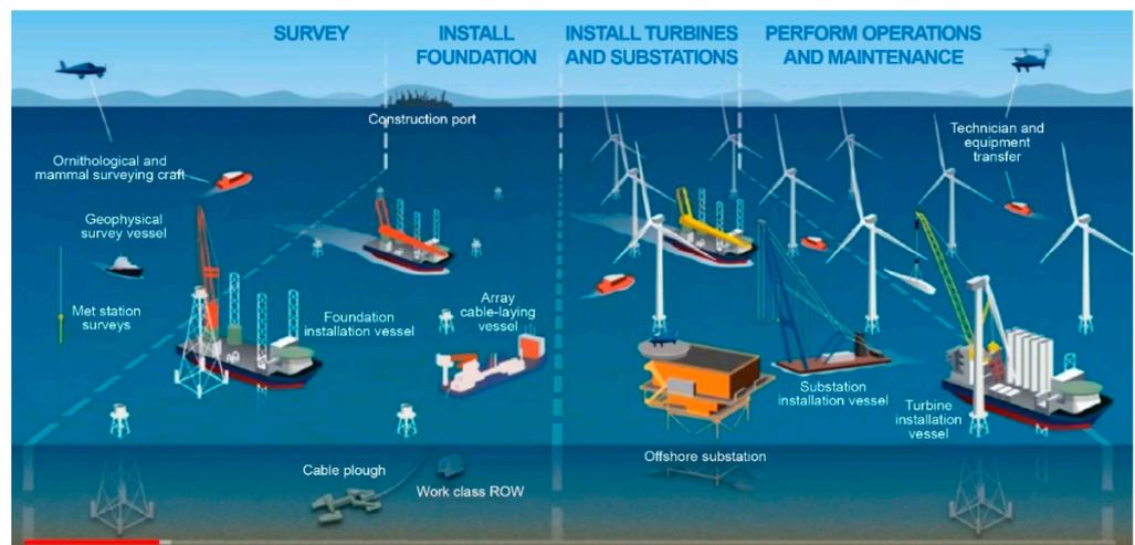
Figure 4. Various offshore vessels used for dedicated purposes at each construction stage (source: Clean Energy Group, Webinar 2019).
