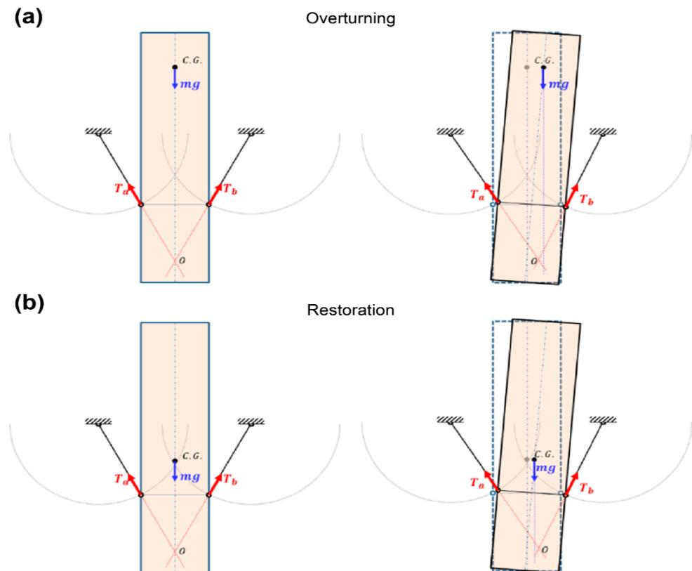
Figure 9. Free-body diagram of a simplified wind turbine.
