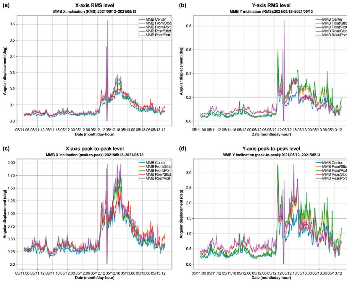
Figure 19. Inclination of the MMB in Case 1.
