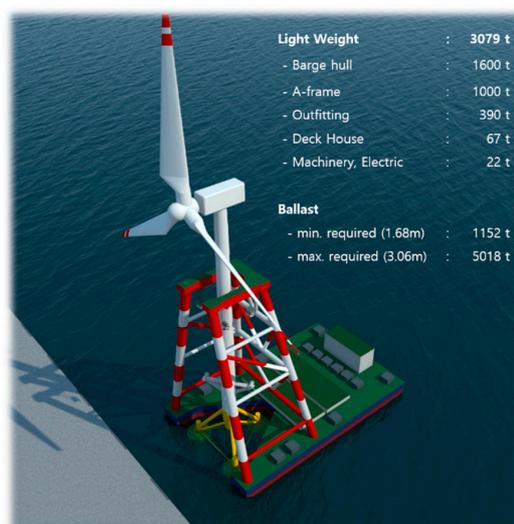
**Figure 14.** Final design of multipurpose mobile base (MMB).
