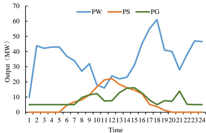
**Figure 3.** The optimized output of wind power, solar power, and natural gas power.
