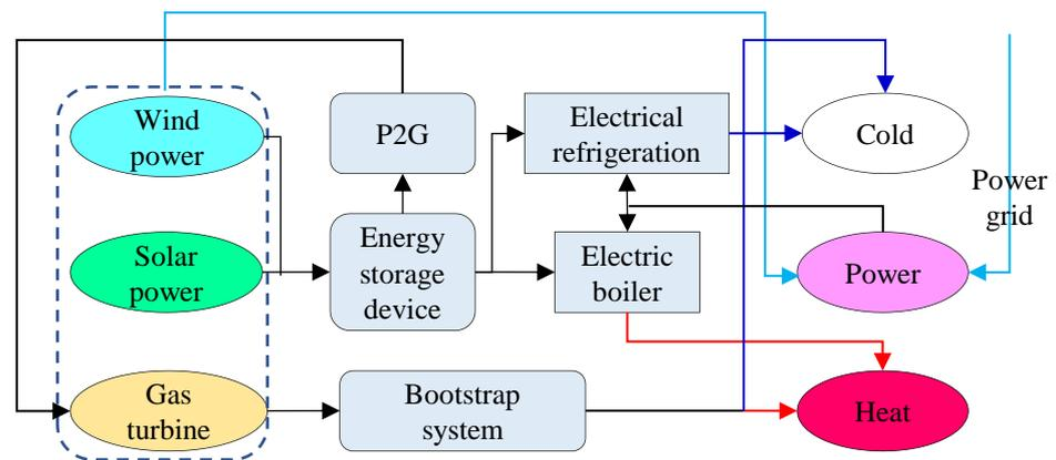
**Figure 1.** Integrated energy system architecture in an industrial park.
