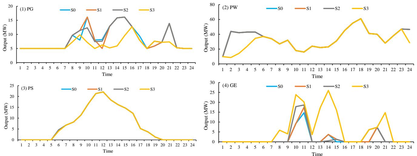
**Figure 5.** The optimized output of gas turbine (1), wind turbine (2), photovoltaic unit (3), and the purchased power (4) amount under different water resource constraints.
