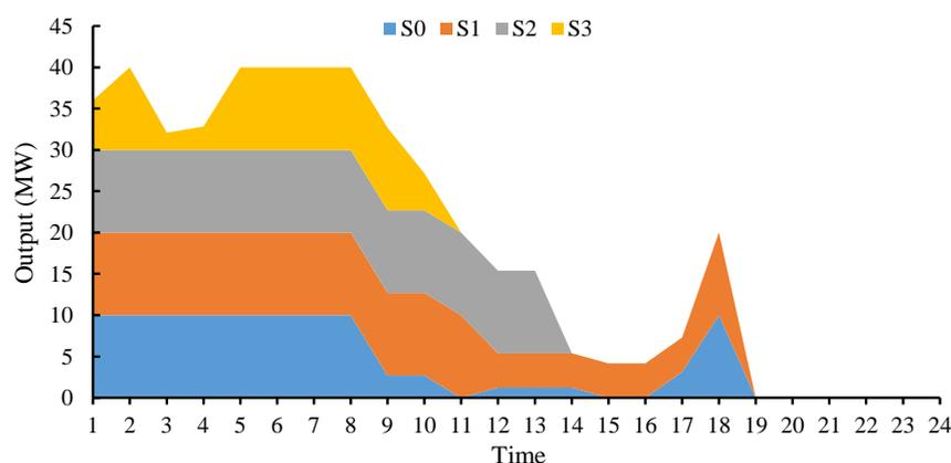
Figure 6. Energy storage amount under different water resource consumption control scenarios.
