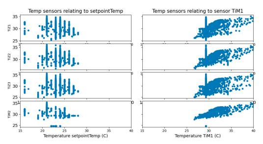
Figure 9. Relationship of temperature sensors, outdoor temperature, and HVAC's set-point.
