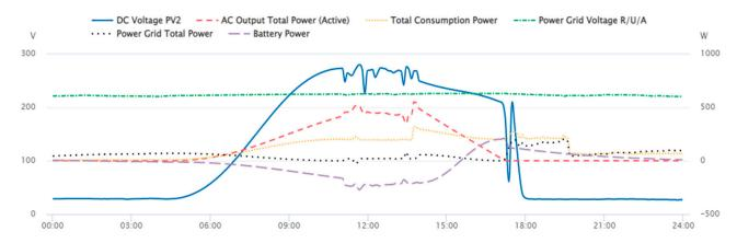
Figure 16. Power flows through inverter in 4 November 2021.
