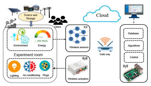
Figure 2. Building monitoring and control system architecture.
