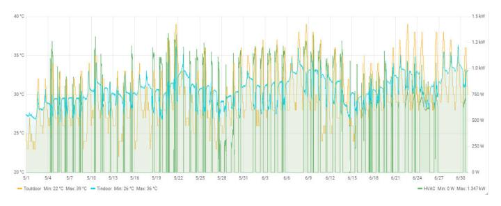
Figure 11. Relationship of HVAC consumption and indoor/outdoor temperature in 1 month.
