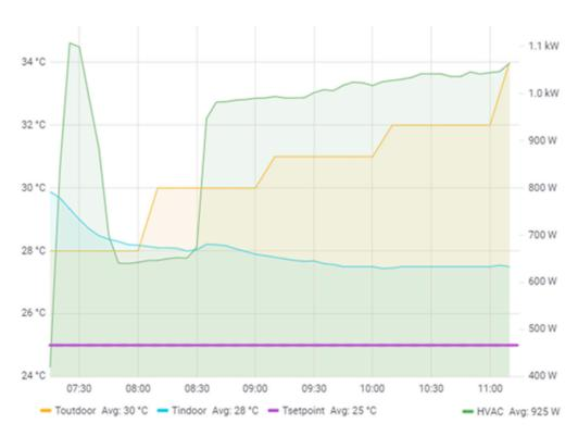
**Figure 13.** Experiment on the second day (Tsetpoint = 25 °C).
