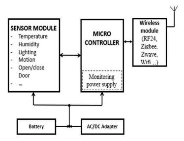
Figure 3. Overview of wireless sensor architecture.
