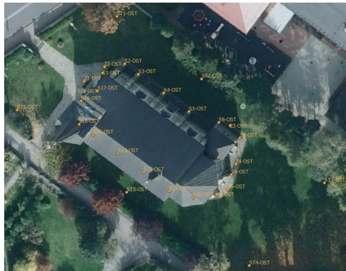
**Figure 4.** Distribution plan of points of the tacheometric and photogrammetric control networks, which also functions as a thermovision control network.
