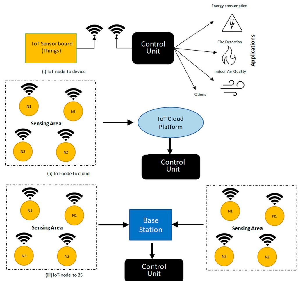
Figure 3. Structures of IoT communication models.
