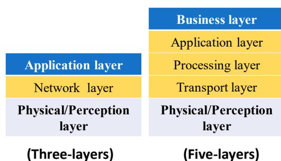
**Figure 1.** IoT architecture with three and five layers.
