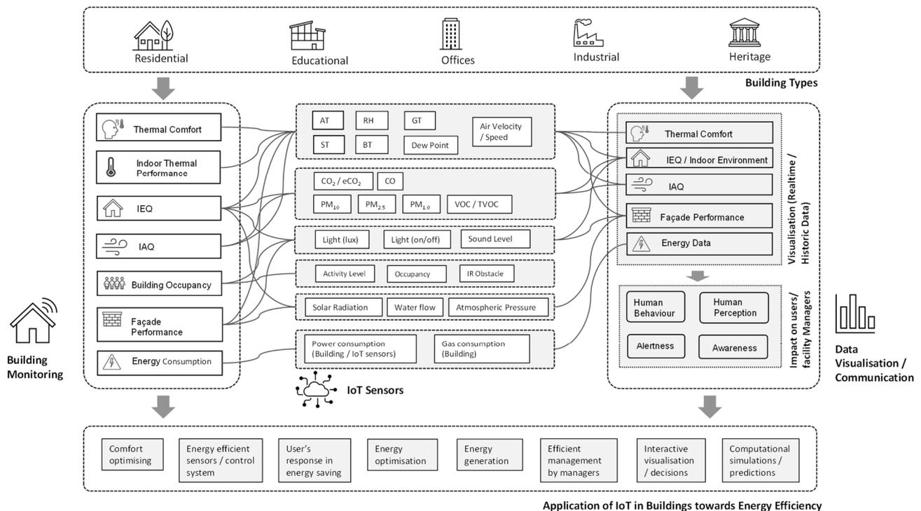
**Figure 10.** Application of IoT sensors in building monitoring and data visualization for energy efficiency.
