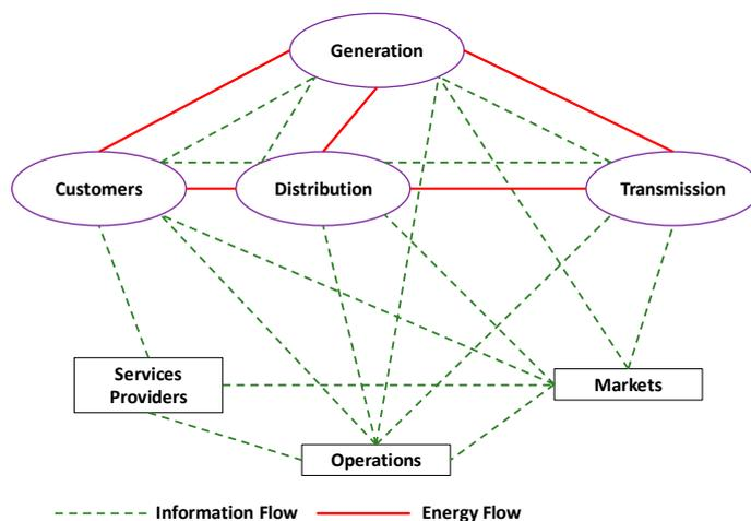
Figure 13. Conceptual model of a smart grid [130].
