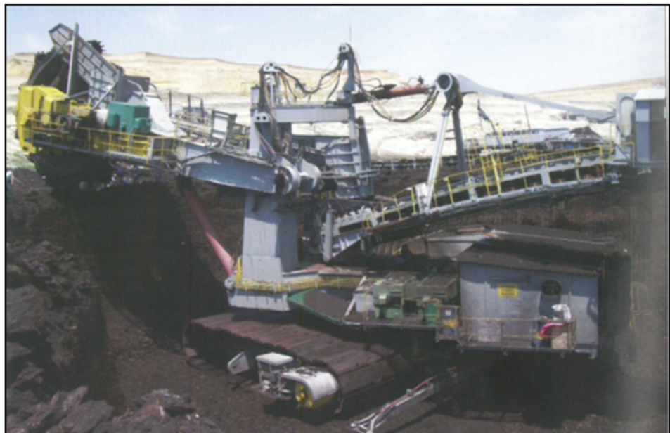
Figure 2. Bucket wheel excavator SRs 400.14/1.5 [19].
