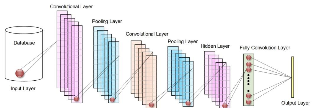
**Figure 6.** General structure of convolutional neural network (CNN) adopted in smart grids.
