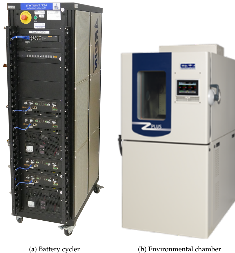
Figure 1. Scientific-grade equipment used to collect OCV characterization data.
