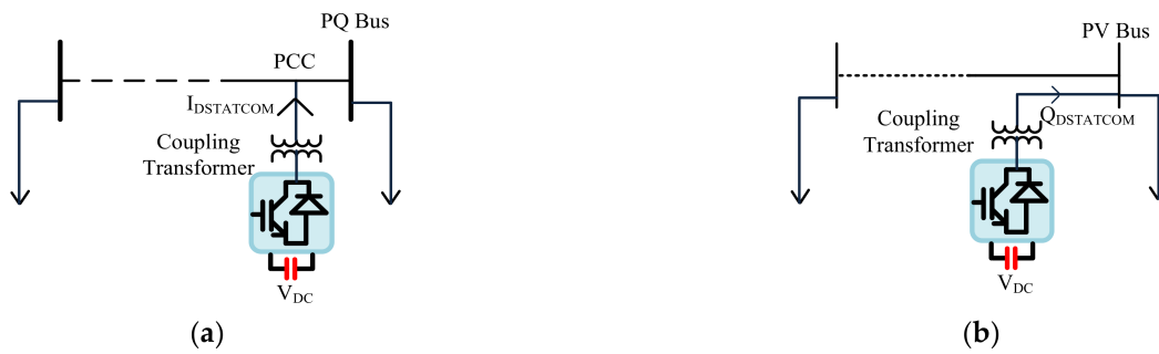
Figure 1. Schematic representation of D-STATCOM modeled as (a) PQ Bus and (b) PV Bus.
