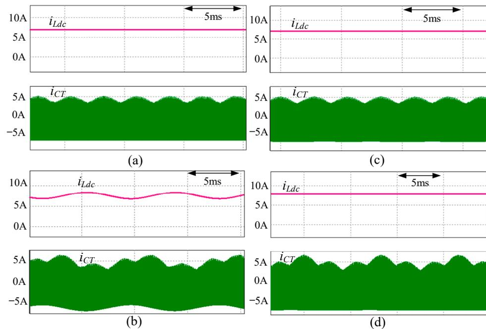
**Figure 11.** The simulated waveforms of the low-voltage-side dc current  $i_{Ldc}$  and the testing capacitor current  $i_{CT}$  for (a,c) balanced and (b,d) unbalanced load conditions in the (a,b) conventional down-scale voltage rating evaluation system, and the (c,d) proposed down-scale voltage rating evaluation system.
