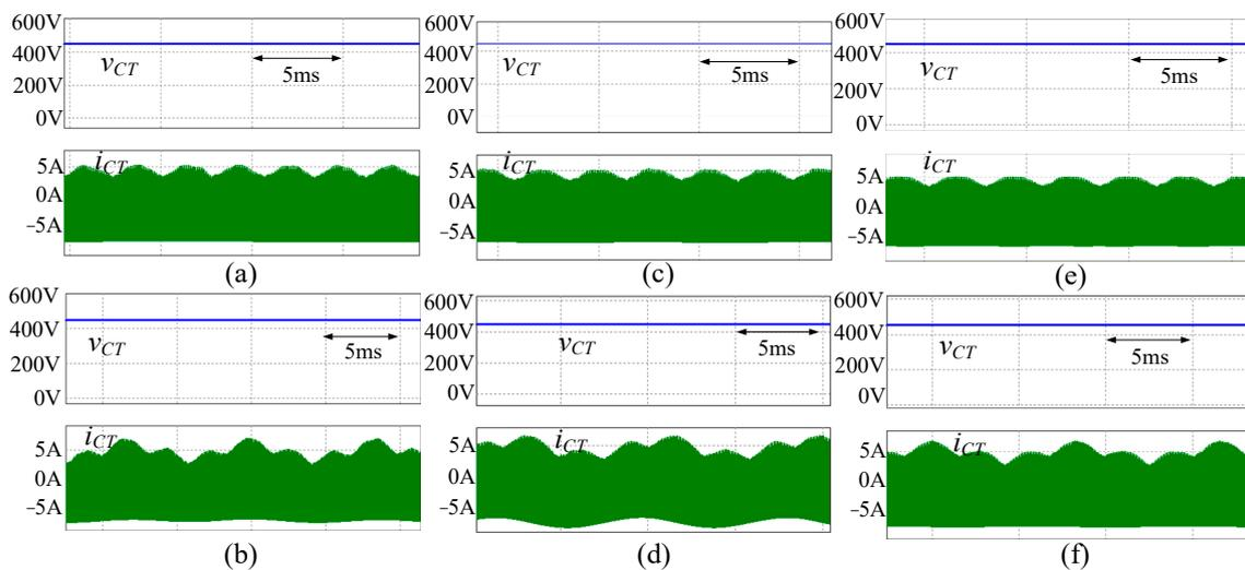
**Figure 8.** The simulated voltage  $v_{CT}$  and current  $i_{CT}$  of the DC-link capacitor under test for (a,c,e) balanced and (b,d,f) unbalanced load condition in the (a,b) full-scale voltage rating VSI, (c,d) conventional down-scale voltage rating evaluation system, and (e,f) proposed down-scale voltage rating evaluation system.
