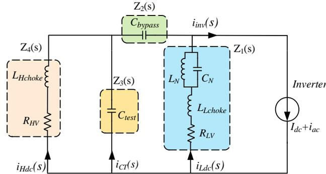
**Figure 4.** Equivalent circuit focusing on the current flowing into the inverter  $i_{inv}$ , capacitor current  $i_{CT}$ , high voltage DC current  $i_{Hdc}$ , and low voltage DC current  $i_{Ldc}$ .
