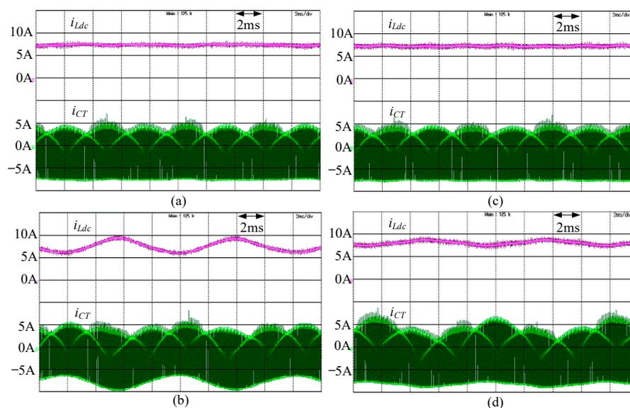
**Figure 13.** The measured waveforms of the low-voltage-side dc current  $i_{Ldc}$  and the testing capacitor current  $i_{CT}$  for (a,c) balanced and (b,d) unbalanced load conditions in the (a,b) conventional down-scale voltage rating evaluation system, and (c,d) proposed down-scale voltage rating evaluation system.
