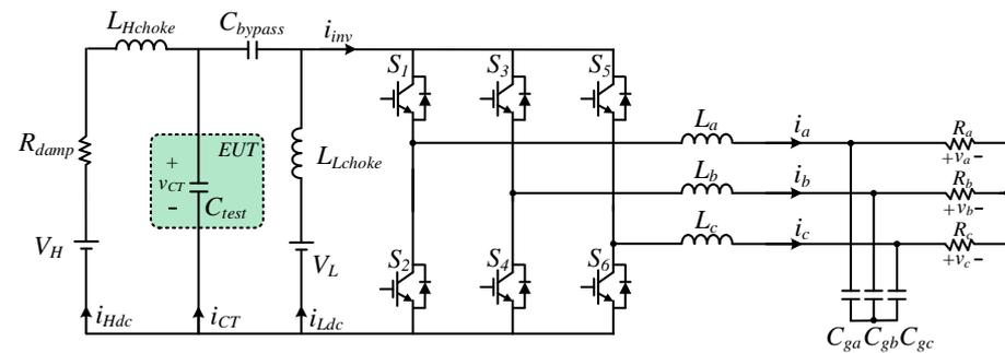
Figure 2. Down-scale voltage rating evaluation system in a high-power three-phase inverter [11].
