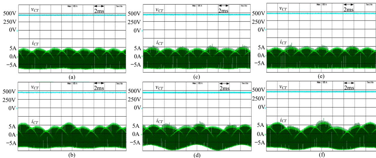
**Figure 12.** The measured voltage  $v_{CT}$  and current  $i_{CT}$  of the DC-link capacitor under test for (a,c,e) balanced and (b,d,f) unbalanced load conditions in the (a,b) full-scale voltage rating VSI, (c,d) conventional down-scale voltage rating evaluation system, and (e,f) proposed down-scale voltage rating evaluation system.
