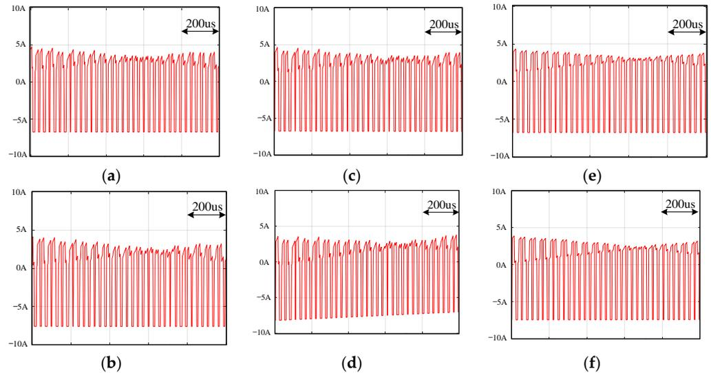
**Figure 9.** The enlarged view of simulated current  $i_{CT}$  of the DC-link capacitor under test for (a,c,e) balanced and (b,d,f) unbalanced load conditions in the (a,b) full-scale voltage rating VSI (c,d) conventional down-scale voltage rating evaluation system, and (e,f) the proposed down-scale voltage rating evaluation system.
