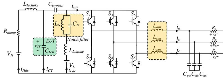
Figure 3. Proposed down-scale voltage rating evaluation system.
