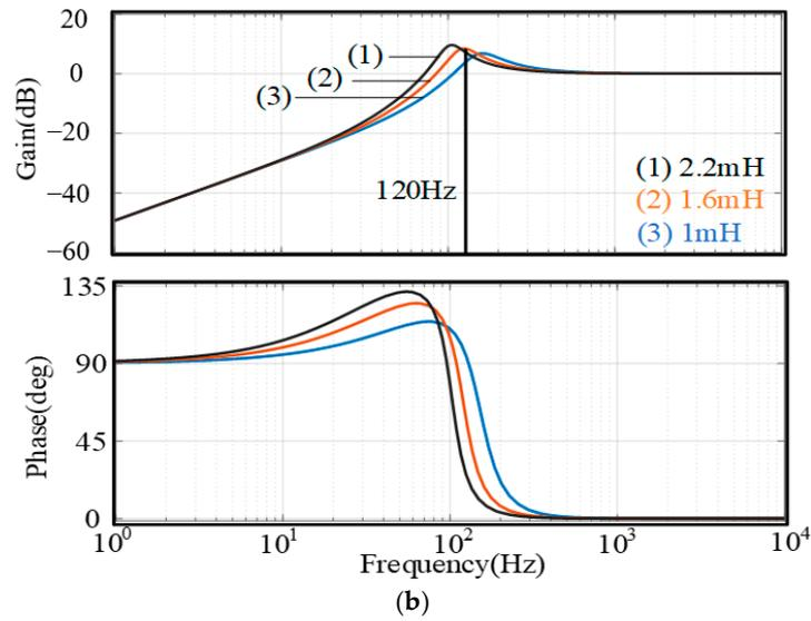
Figure 5. Bode plot of the transfer function in evaluation system proposed in [11]. (a)  $G_3(s)$ . (b)  $G_4(s)$ .
