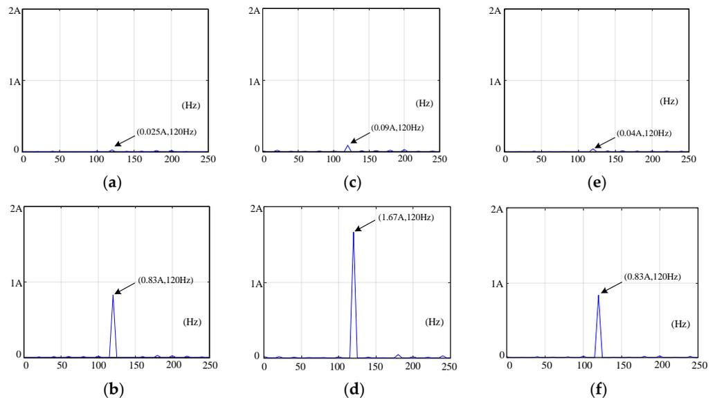
**Figure 10.** Close-to-120 Hz FFT results of current  $i_{CT}$  of the DC-link capacitor under test for (a,c,e) balanced and (b,d,f) unbalanced load conditions in the (a,b) full-scale voltage rating VSI, (c,d) conventional down-scale voltage rating evaluation system, and (e,f) proposed down-scale voltage rating evaluation system.
