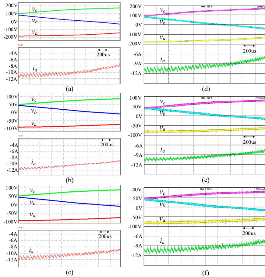
**Figure 7.** Simulation (left) and corresponding experimental (right) waveforms of output three-phase voltages  $V_a$ ,  $V_b$ ,  $V_c$  and output current  $i_a$  under (a,d) full-scale VSI with output inductor 2 mH, (b,e) conventional down-scale voltage rating evaluation system with output inductor 2 mH, and (c,f) proposed down-scale voltage rating evaluation system with output inductor 1 mH.
