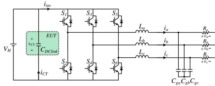
Figure 1. Full-scale voltage rating evaluation system in a high-power three-phase inverter.
