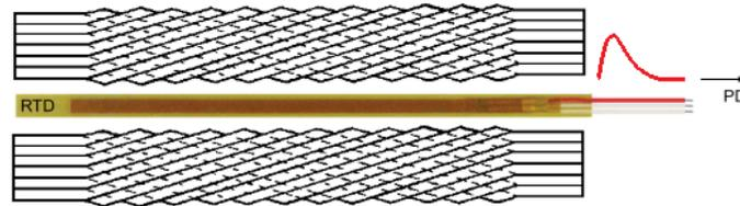
Figure 24. RTD allocated in the slot, adapted from [98].
