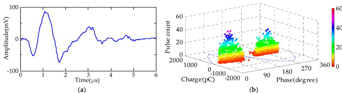
**Figure 6.** Data (a) waveform, (b) PRPD pattern [13].
