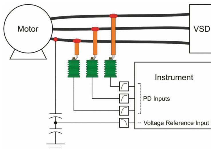
**Figure 23.** Structure of the PD measurement system [95].
