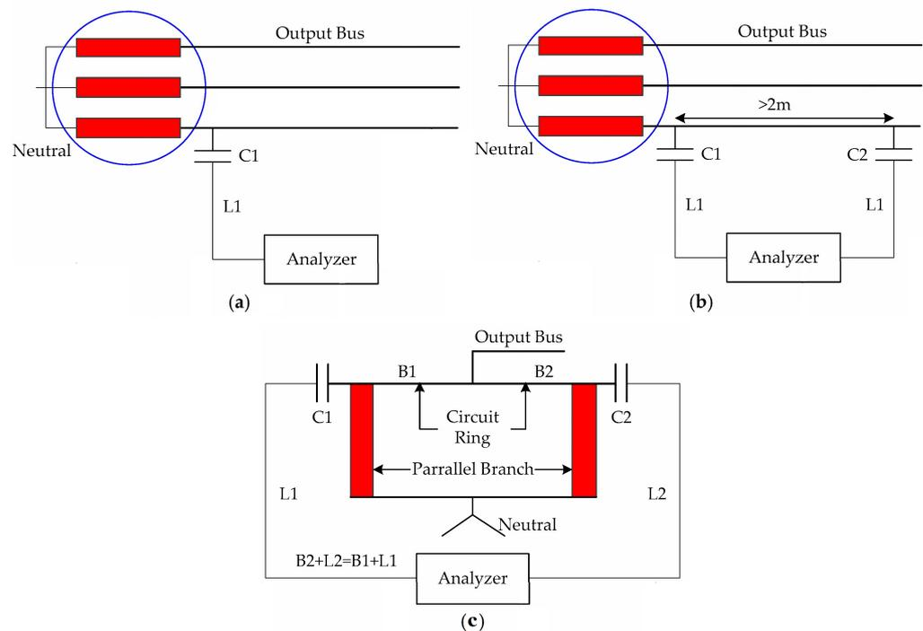
**Figure 4.** Configurations (a) simple, (b) directional and (c) differential, adapted from [13].
