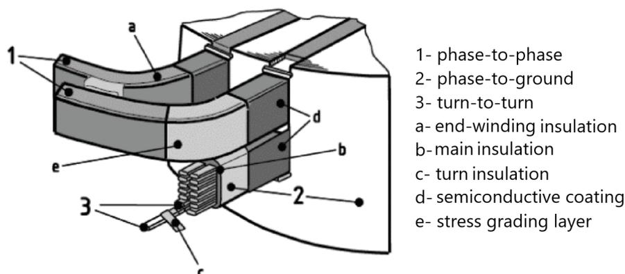
**Figure 2.** Preformed stator winding, adapted from [16].
