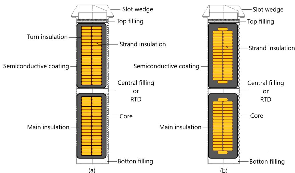
**Figure 1.** Cross-section of a slot (a) multi-turn coil and (b) Roebel bar.
