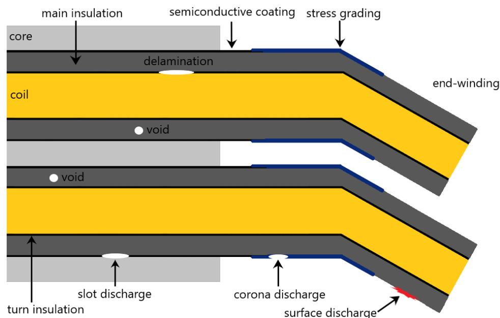
**Figure 3.** PD sources in the isolation system of a typical machine.
