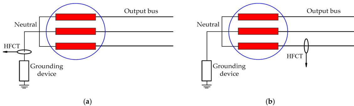
**Figure 5.** Configurations (a) neutral ground connection, (b) terminal, adapted from [13].
