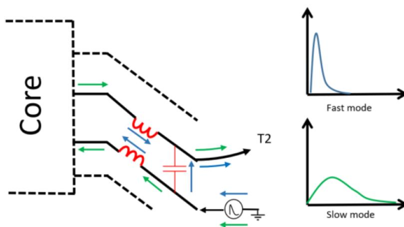
Figure 17. Capacitive and inductive coupling between bus [28].
