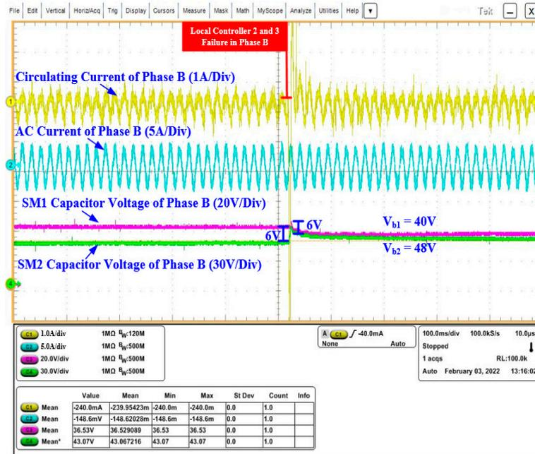
Figure 19. System parameters under failure of two local controllers.
