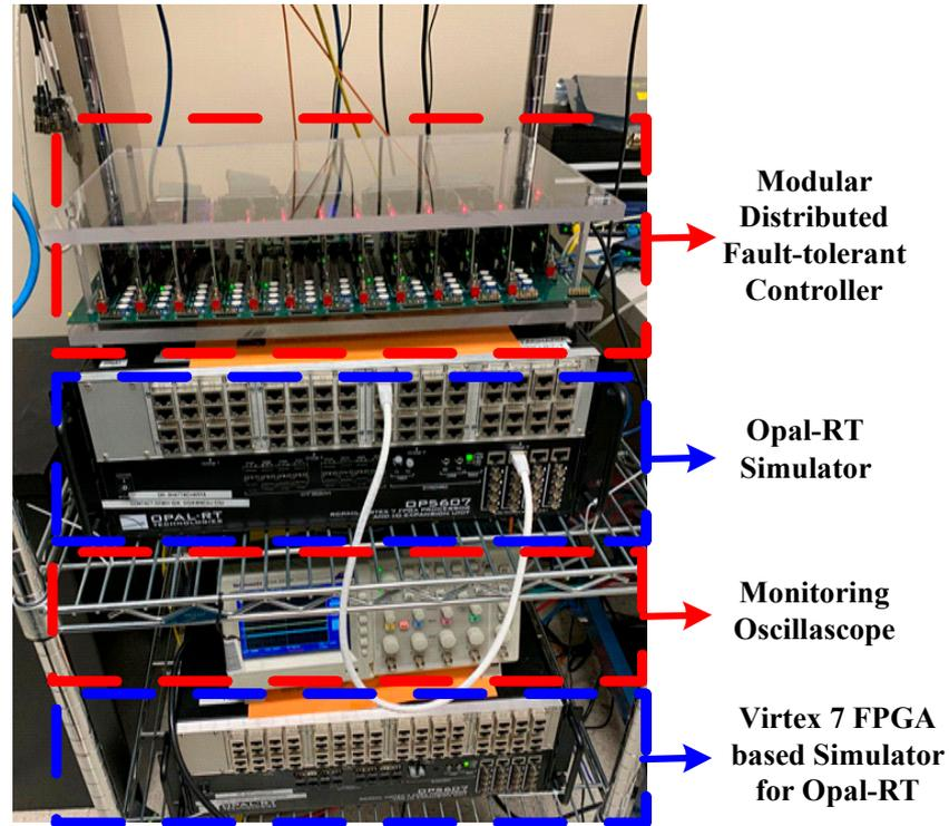
Figure 20. Opal RT and the controller HIL setup.
