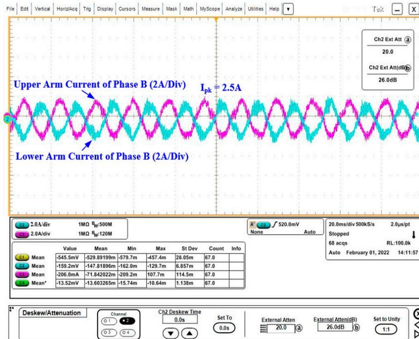
Figure 16. Arm Currents of phase B under steady state.
