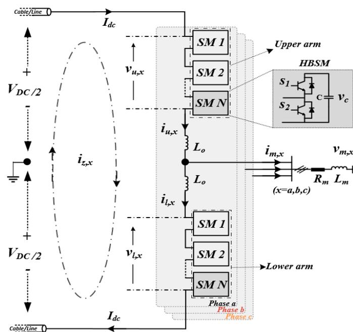
Figure 1. Three-phase MMC circuit with HBSM configuration.
