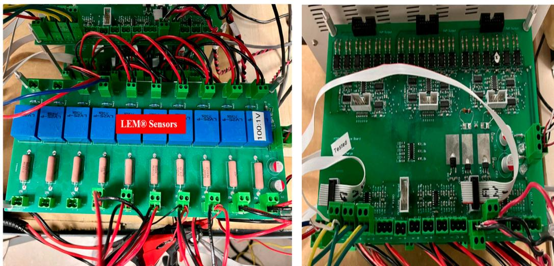
**Figure 13.** Sensor (left) and signal conditioning (right) board of the MMC prototype.
