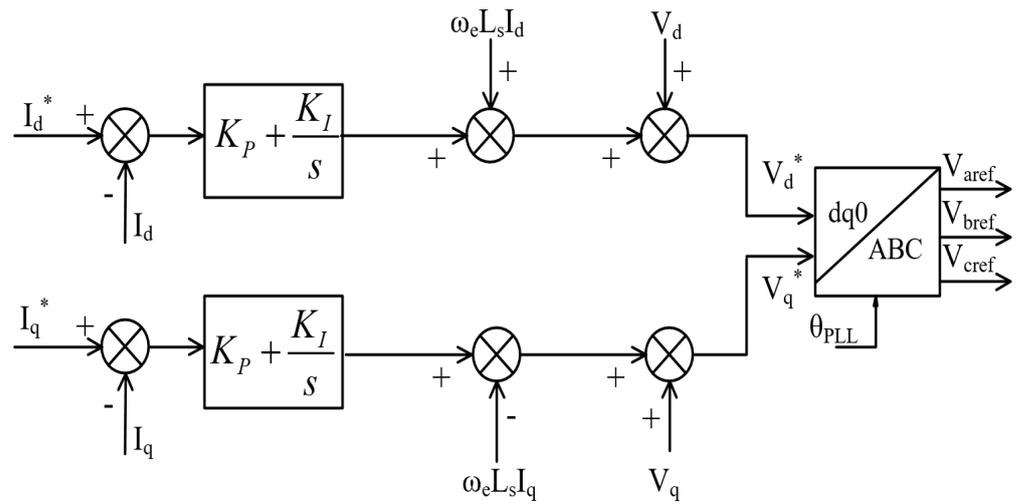
Figure 8. A block diagram of the implemented voltage controller.
