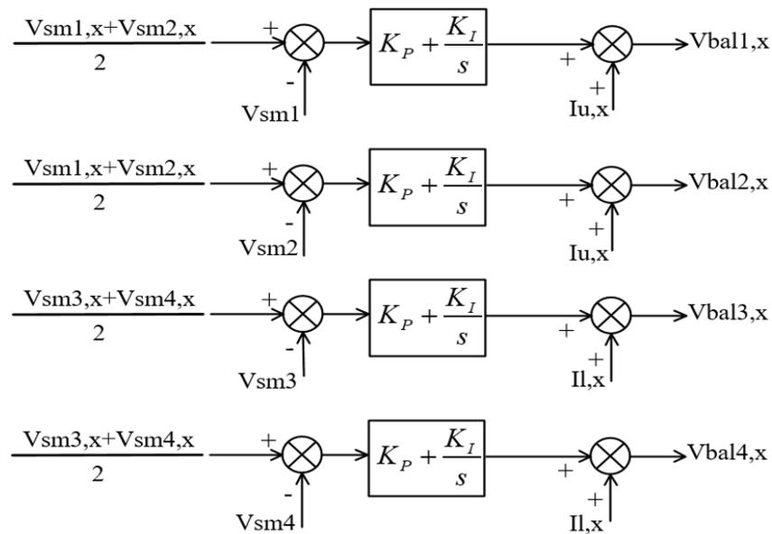
Figure 9. A block diagram of the implemented SM capacitor voltage balancing controller.
