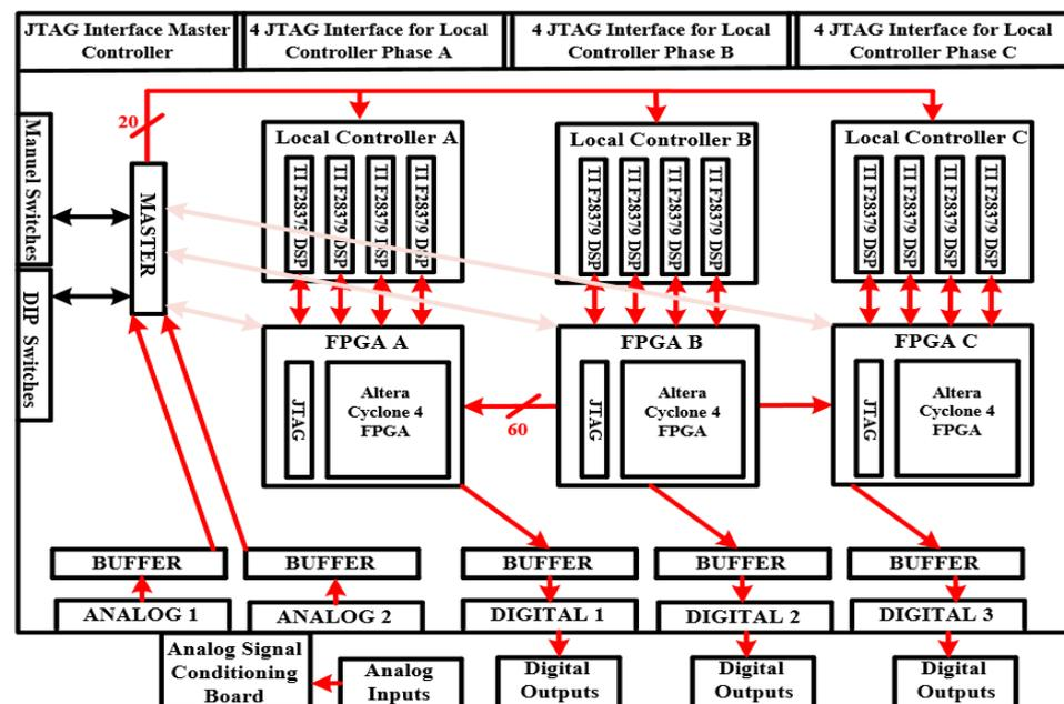
Figure 5. A block diagram of the controller.
