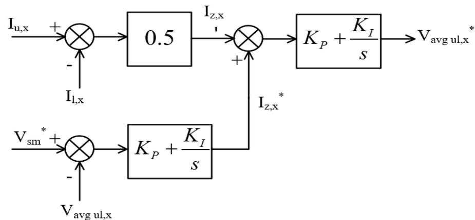
Figure 3. A block diagram of the implemented phase averaging controller.
