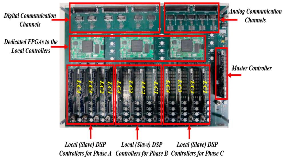
Figure 4. Modular distributed fault-tolerant controller.
