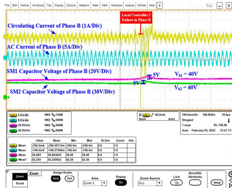
Figure 18. System parameters under failure of one local controller.
