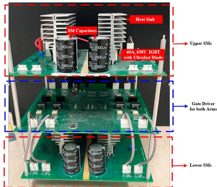
**Figure 12.** A phase leg of the MMC prototype.
