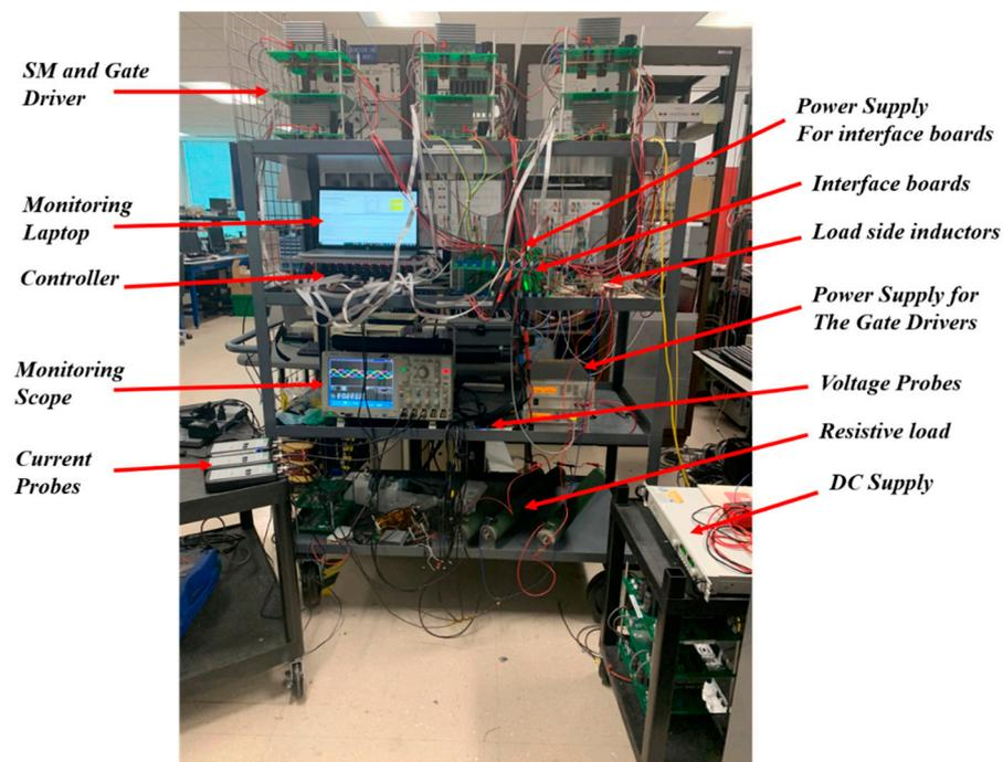
Figure 11. A photo of the test-setup with MMC prototype and the controller.
