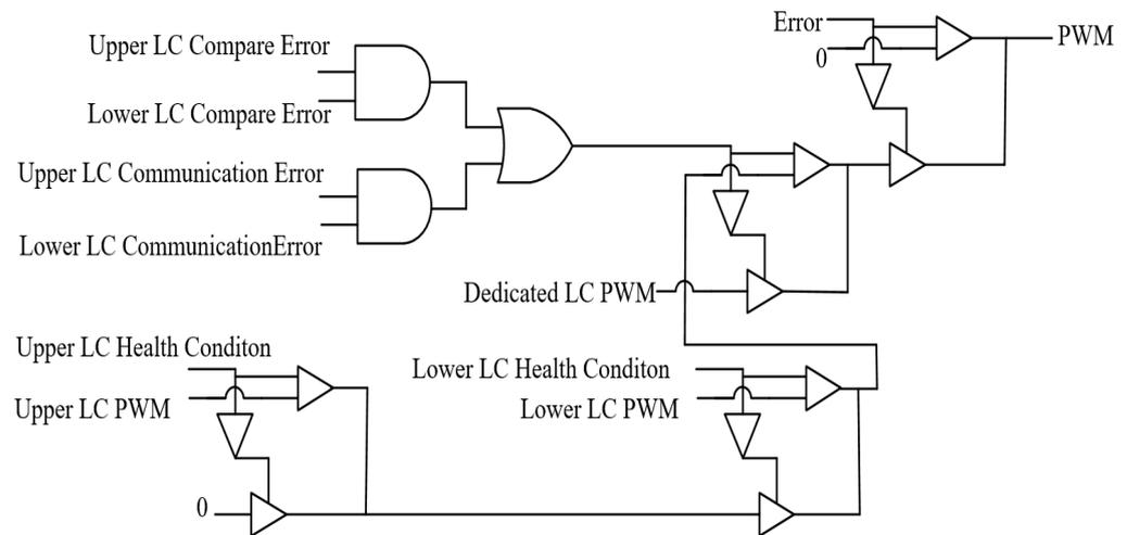
**Figure 6.** A logic diagram of the SM controller failure detection.
