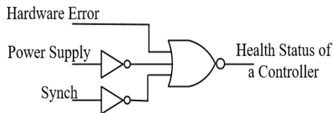
**Figure 7.** A logic diagram of the health status check controller.
