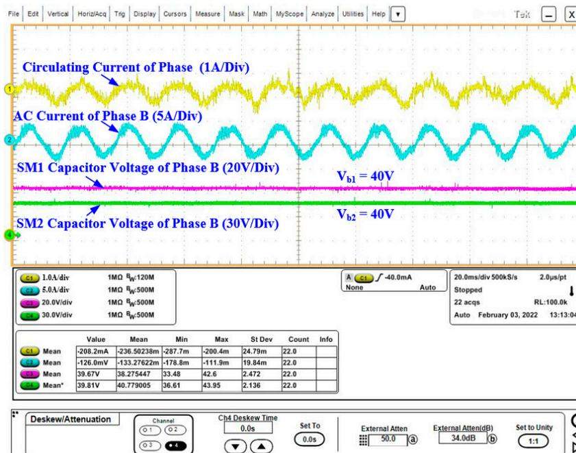
Figure 17. Parameters of phase B under steady state.
