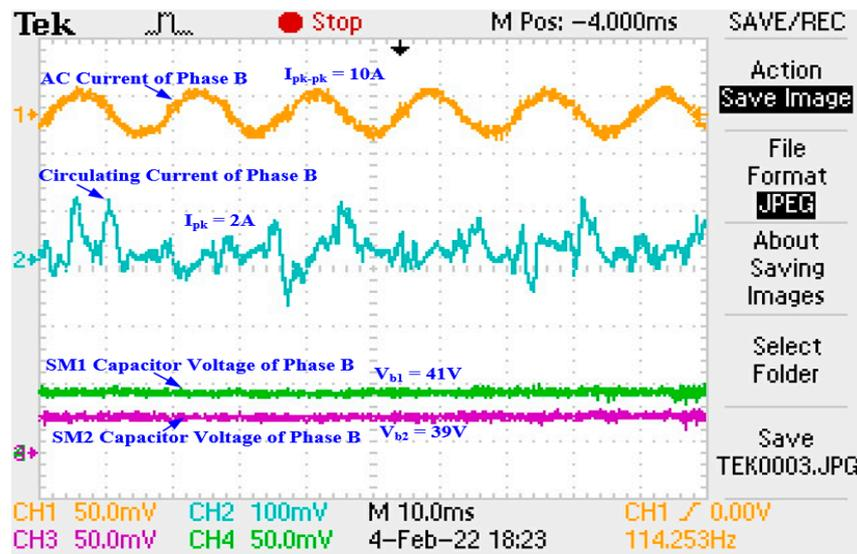
Figure 21. Result validation of Figure 17 with Opal-RT.
