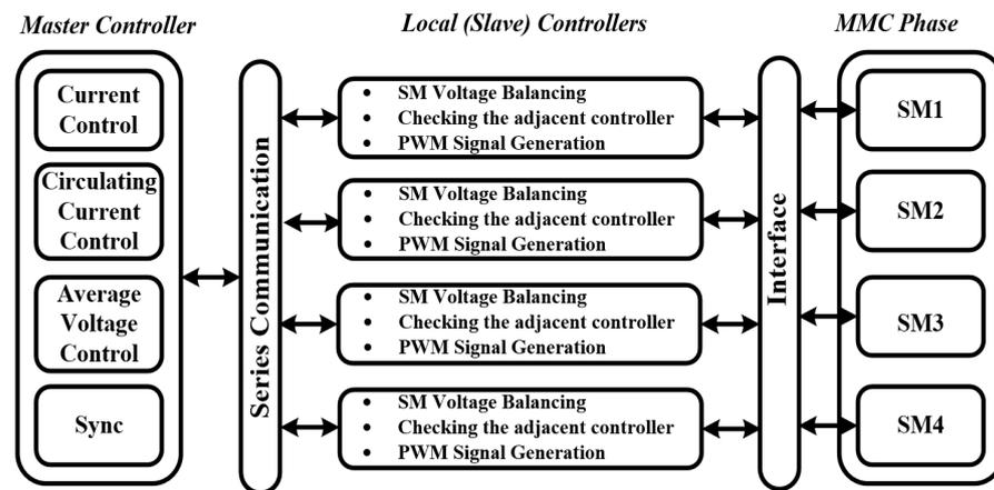
Figure 2. An illustration of the modular distributed fault-tolerant controller.
