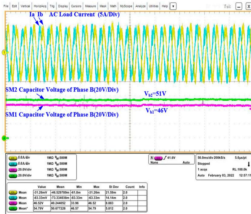
Figure 15. AC current and SM capacitor voltage at 100 V DC link.
