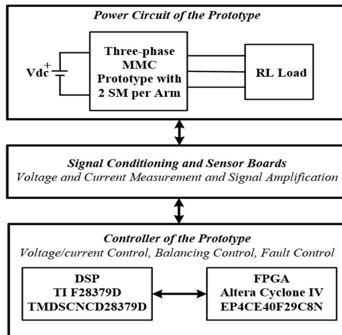
Figure 10. An illustration of the test-setup.
