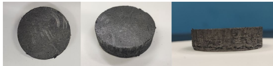
Figure 2. Photos of n-tetradecane/EG composite.
