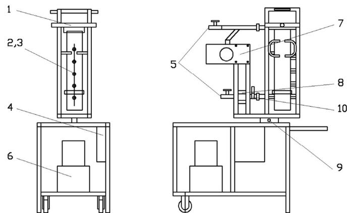
**Figure 4.** Laboratory test device structure (1—gas generator; 2,3—temperature probes; 4—electric panel; 5—pneumatic throttles; 6—compressor; 7,8—air flow meters; 9—electronic scale; 10—pressure transducer. The same components—in their physical form—are shown in Figure 5b below).
