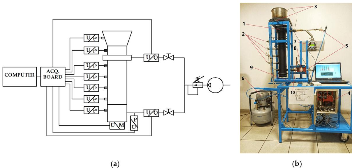
**Figure 5.** Test device in our laboratory: (a) functional diagram; (b) physical embodiment (1—gasifier; 2—pyrolytic front temperature probes; 3—water and flame temperature probes; 4—electric panel; 5—pneumatic throttles; 6—compressor; 7—combustion air flowmeter; 8—pyrolysis air flowmeter; 9—electronic scale; 10—pressure transducer) [25].
