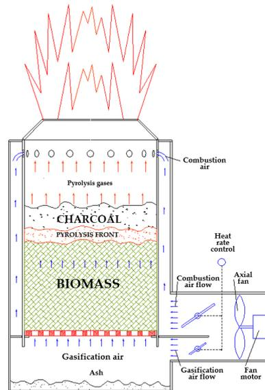
**Figure 1.** Functional diagram of the gasifier working on the Top-Lit Updraft (TLUD) principle [13].
