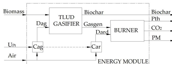
Figure 3. Block diagram of the TLUD energy module [13].
