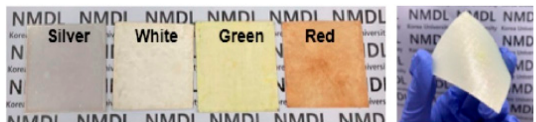
Figure 33. White, green, and red colored DPRC emitter for sub-ambient cooling [161].
