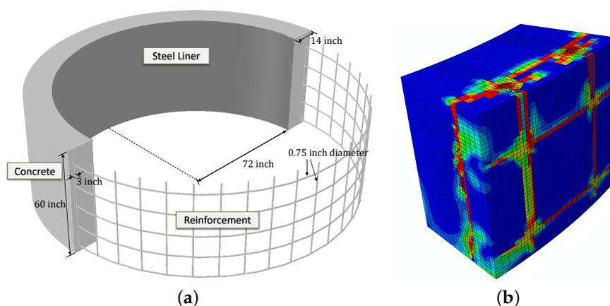
**Figure 3.** FEM of concrete ring structure [63]. (a) concrete ring structure; (b) degradation in model.
