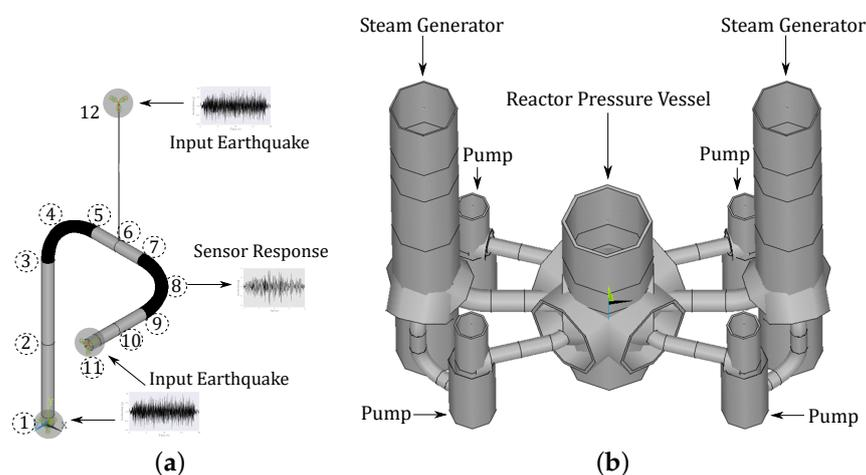
**Figure 1.** Nuclear piping-equipment systems [56]. (a) piping system 1; (b) piping system 2.
