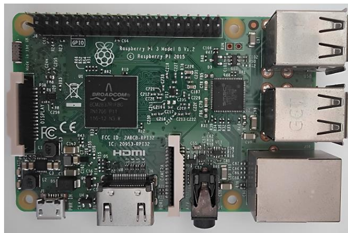
Figure 5. The Raspberry Pi 3 model B used to realize the proposed home gateway.
