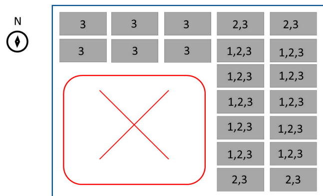
Figure 3. Diagram of the arrangement of PV panels on the water intake plot (1—PV 3.0 kW variant, 2—PV 4.2 kW variant, 3—PV 6.0 kW variant).
