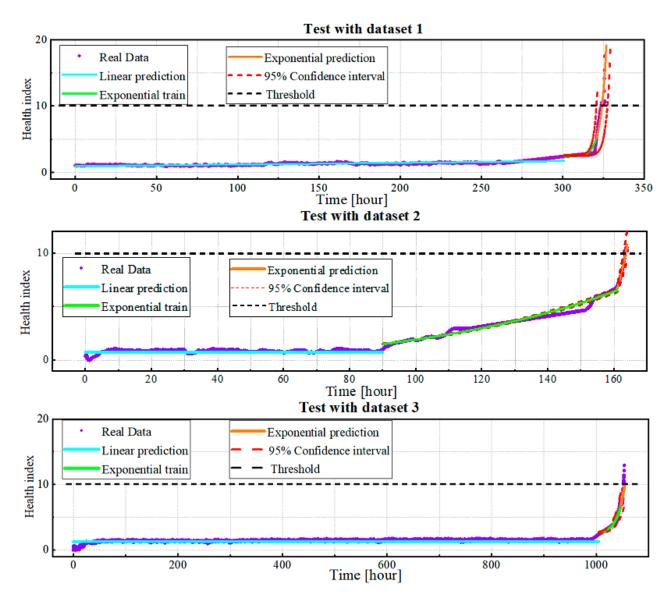
Figure 11. RUL prediction results of degradation models.
