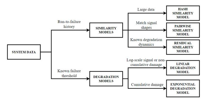
Figure 8. Approach to predicting RUL of main bearing.
