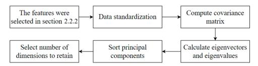
Figure 3. The process of determining HI from PCA.
