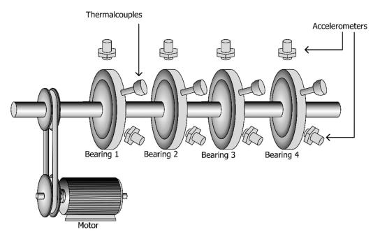
Figure 1. Bearing test rig.
