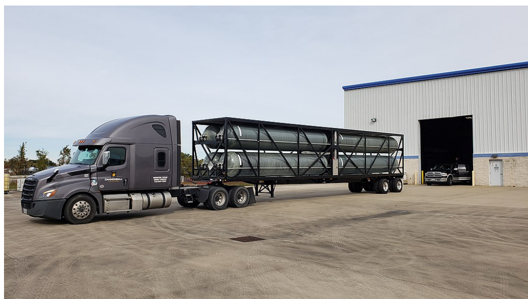
Figure 22. Tube trailers for pressurised hydrogen gas transportation [136].
